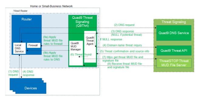
The messages that are exchanged among architectural components to support threat signaling are depicted by arrows and numbered in sequence in Figure 7-2. The result of this message flow is to protect a local device from connecting to a domain that has been identified as unsafe by a threat intelligence service from which Quad9 DNS service receives information which, in this case, is ThreatSTOP.
