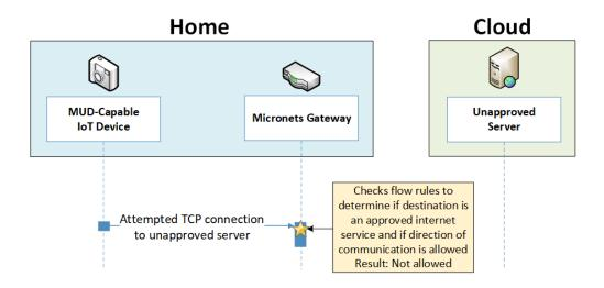
Figure 8-7 Unapproved Communications Message Flow—Build 3
