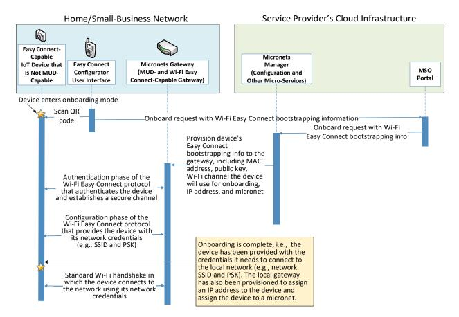
Figure 8-5 Non-MUD-Capable IoT Device Onboarding Message Flow—Build 3
