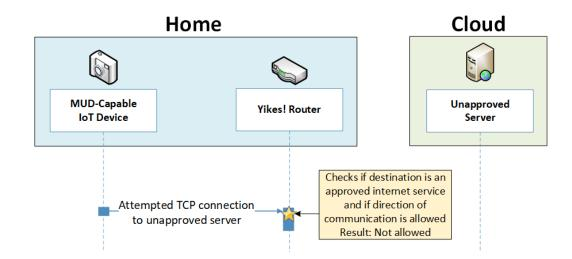
Figure 7-7 Unapproved Communications Message Flow—Build 2
