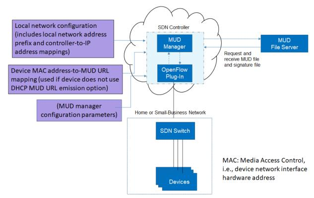
As shown in Figure 9-2, the MUD manager exports a YANG-based REST API to allow administrators to configure the SDN controller/MUD manager. This API is not exposed to the network users. It provides the following capabilities:
