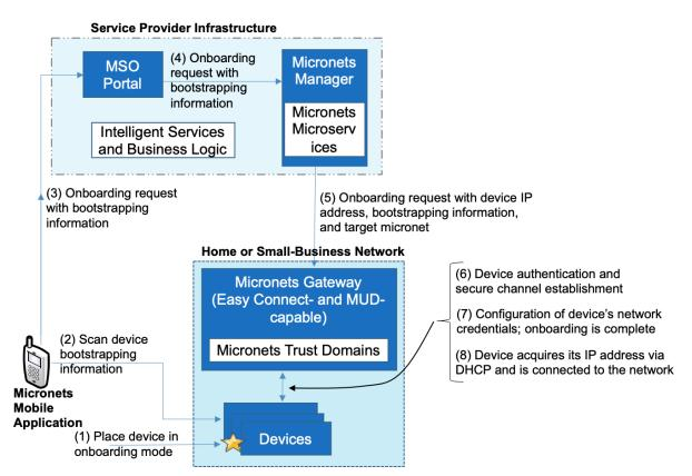
As shown in Figure 8-2, the flow of messages needed to support onboarding a non-MUD-capable device in Build 3 is as follows:
