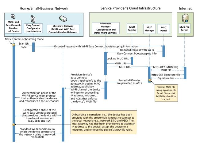
The components used to support Build 3 are deployed across the home/small-business network, the service provider cloud, and the internet in general. As shown in Figure 8-4, the onboarding message flow for MUD-capable devices is as follows:
