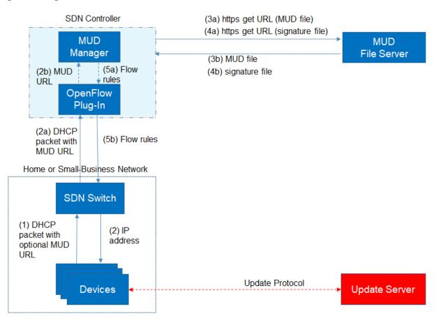
As shown in Figure 9-1, the steps that occur when a MUD-capable IoT device connects to the home/small-business network using Build 4 are as follows:
