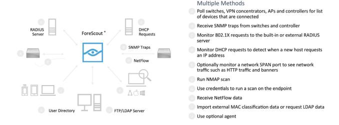
Forescout is deployed as virtual appliances on the NCCoE laboratory network and managed by a single enterprise manager. After discovering IoT devices and collecting relevant information, classification is the next step.
