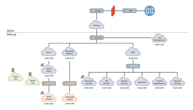
Figure 4-6 Network Segmentation and VLAN Within the RPM Lab
