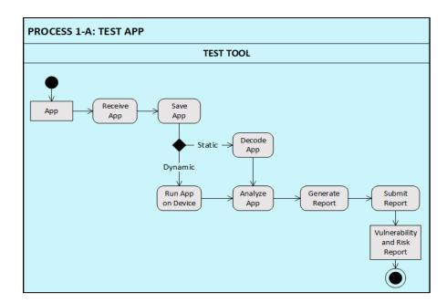
Figure 5 - Test tool workflow.
