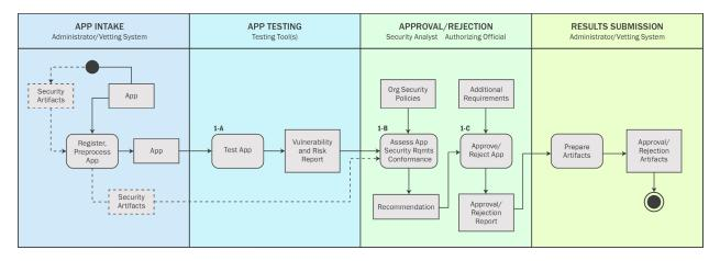
Figure 4 - Four sub-processes of an app vetting process.
