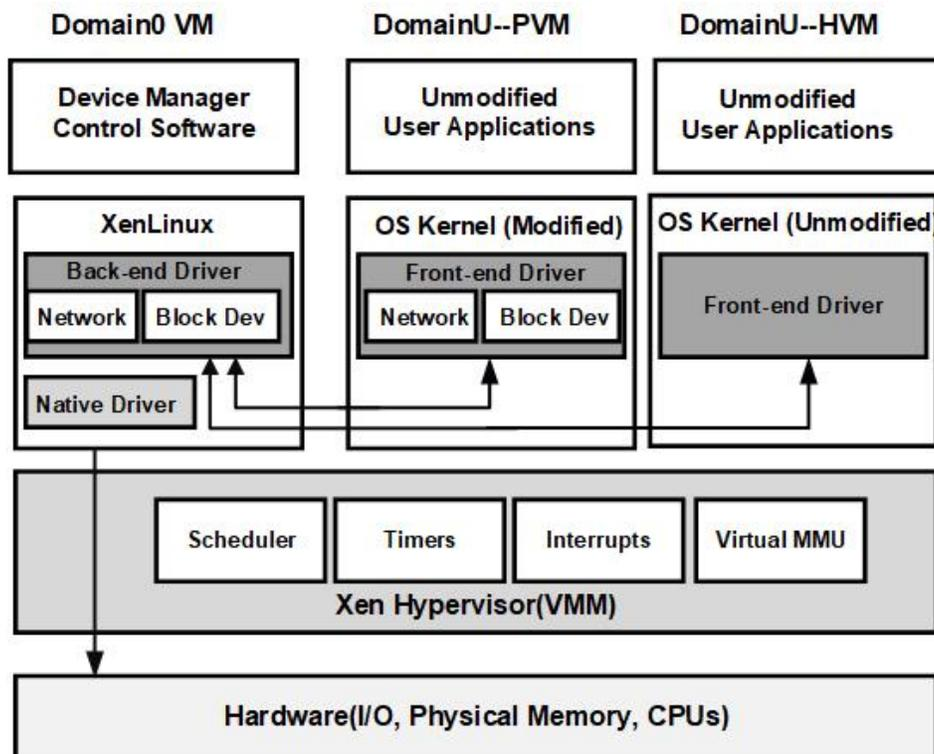
Figure 1: The Xen architecture
