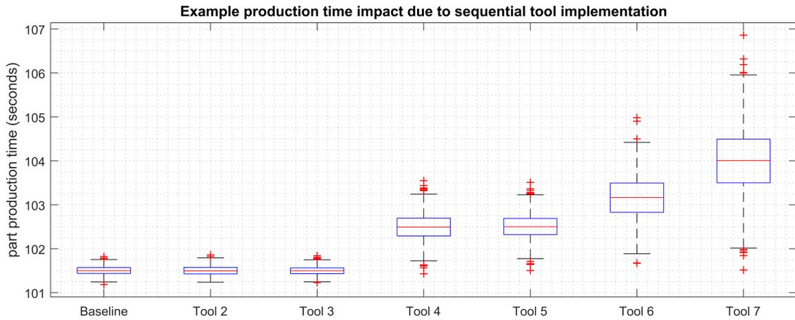
**Fig. 6.** An example box plot illustrating how increasing performance degradation of a manufacturing system may appear as tools are sequentially added to the system.
