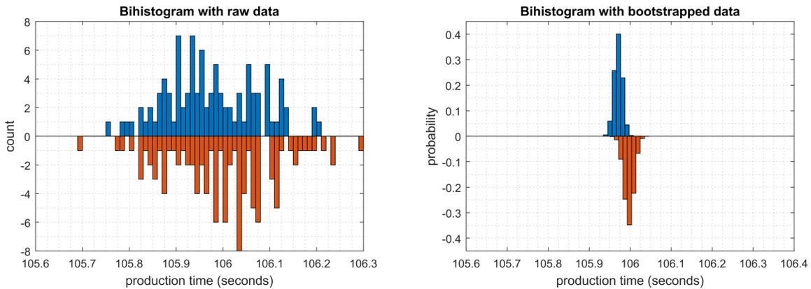
**Fig. 5.** Example bihistograms of production data. The first bihistogram uses raw production data, while the second uses bootstrapped production data.
