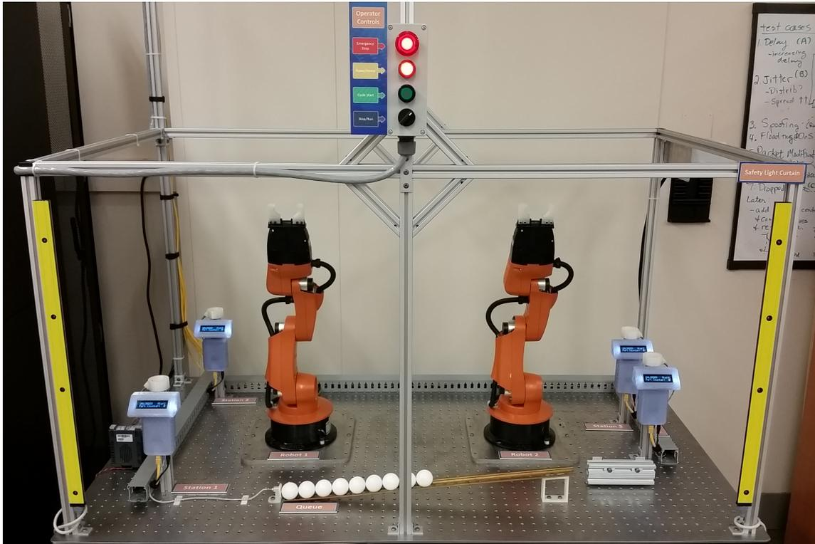
**Fig. 1.** The CRS workcell in standby, waiting for the operator to initiate the manufacturing process. The operator control panel is visible at the top of the figure.
