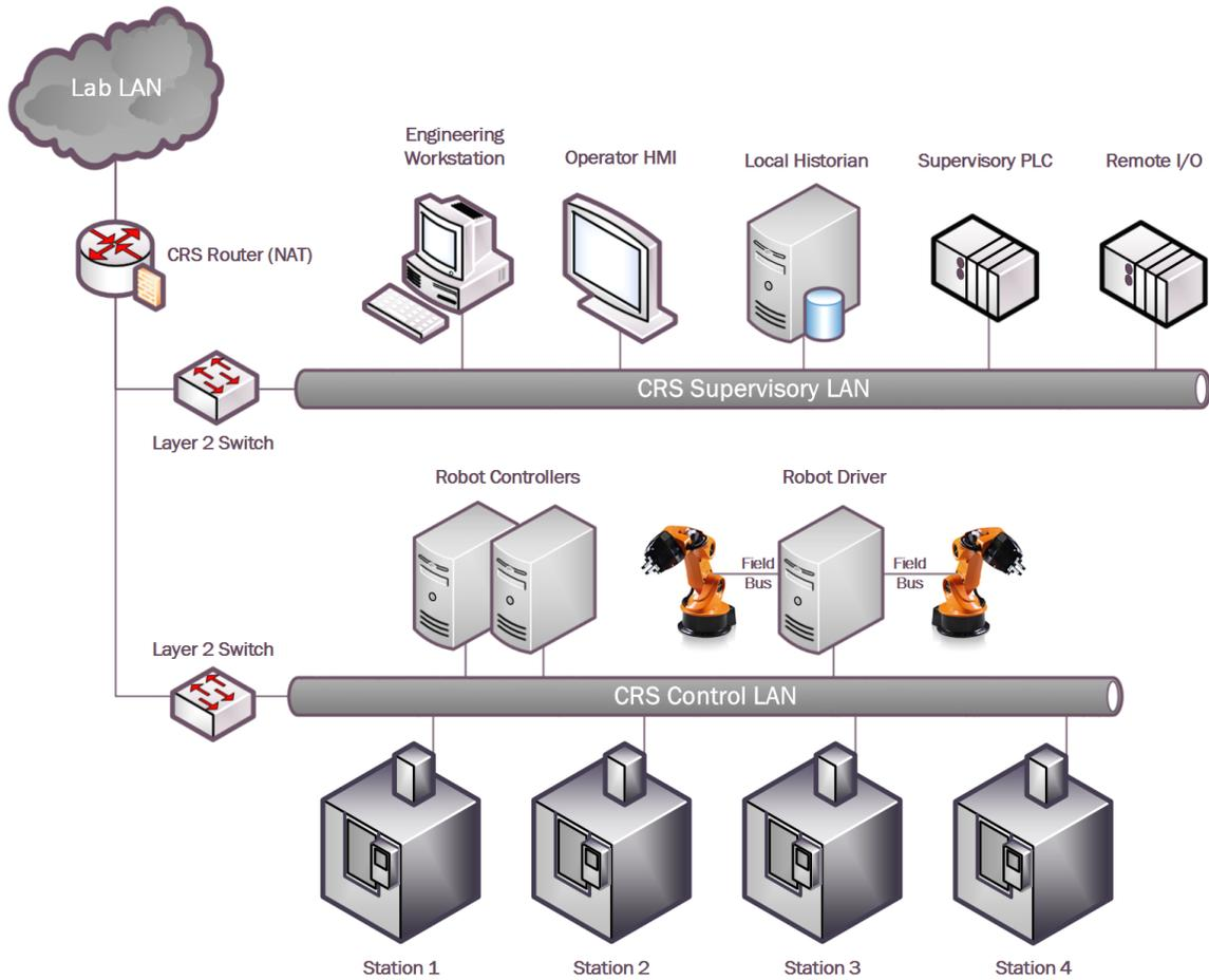
**Fig. 4.** Network topology diagram of the CRS.
