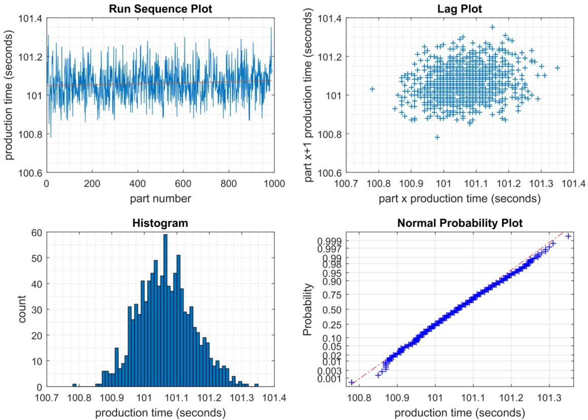
**Fig. 8.** Four plot of the ‘part production time’ KPI from parts produced during workcell characterization.
