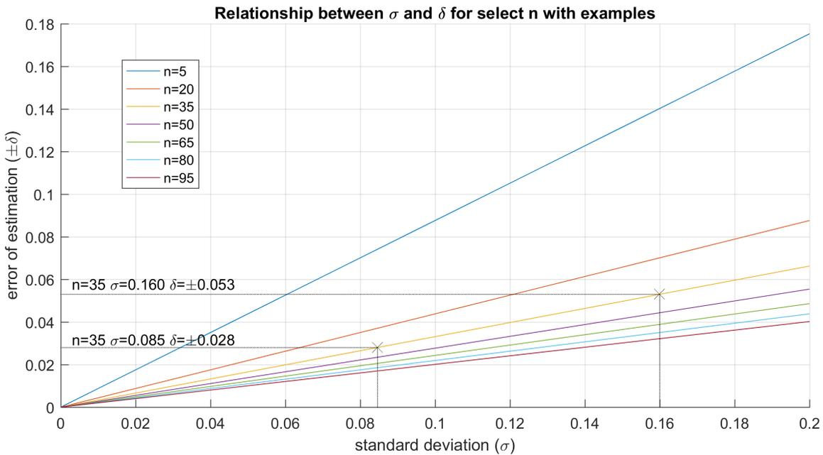
**Fig. 12.** Plot displaying the relationship between the standard deviation  $\sigma$ , error of estimation  $\delta$ , and sample size  $n$ . The two examples shown demonstrate the increasing error of estimation as the standard deviation of the manufacturing process becomes larger. In this case, an increase of  $\sigma$  to 0.160 causes  $\delta$  to increase to  $\pm 0.053$ , much larger than the characterized  $\delta$  of  $\pm 0.028$ .
