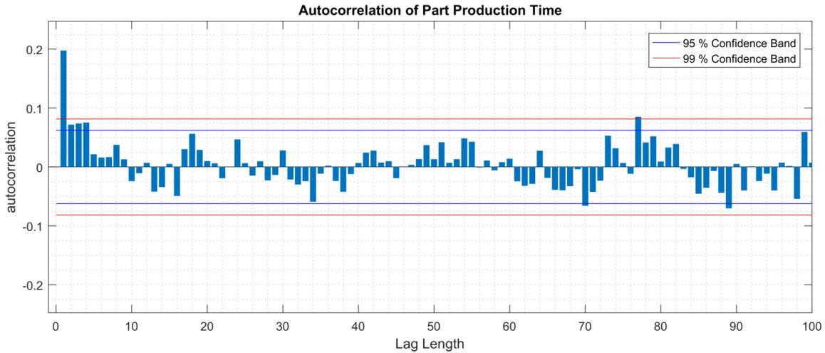
**Fig. 9.** Autocorrelation plot showing lag 1 to lag 100 of the production time KPI.
