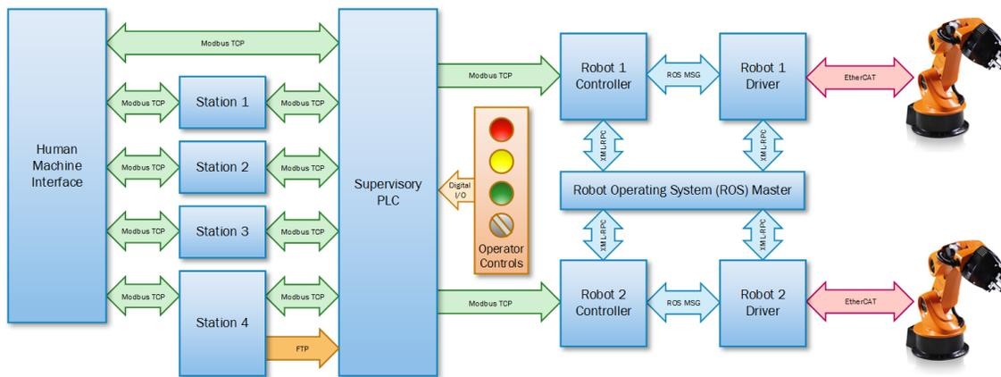
**Fig. 3.** Data flows between workcell subsystems and their respective network protocols, as required for normal manufacturing operations.
