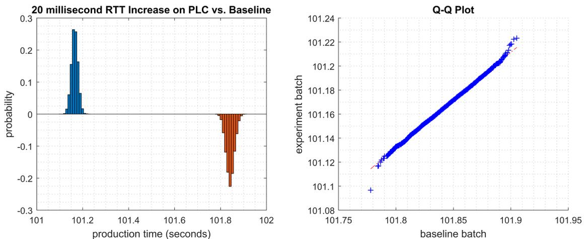
**Fig. 13.** Bihistogram showing the production time probability of the baseline measurements (blue-colored histogram) and the post-implementation measurements (orange-colored histogram).
