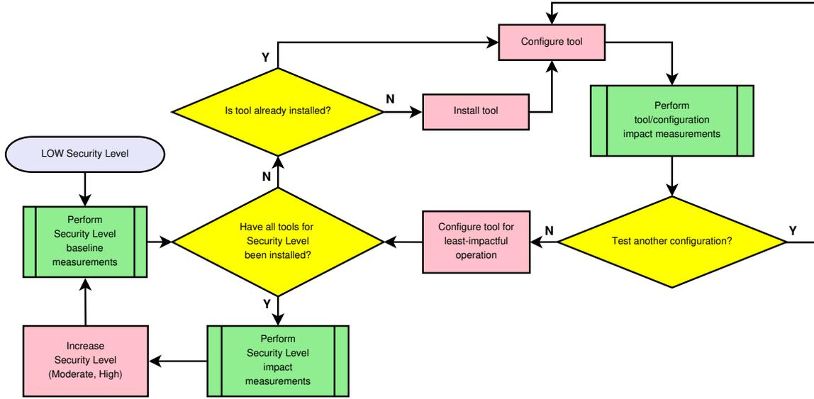
**Fig. 2.** Flow chart describing the implementation process for all Manufacturing Profile security levels.
