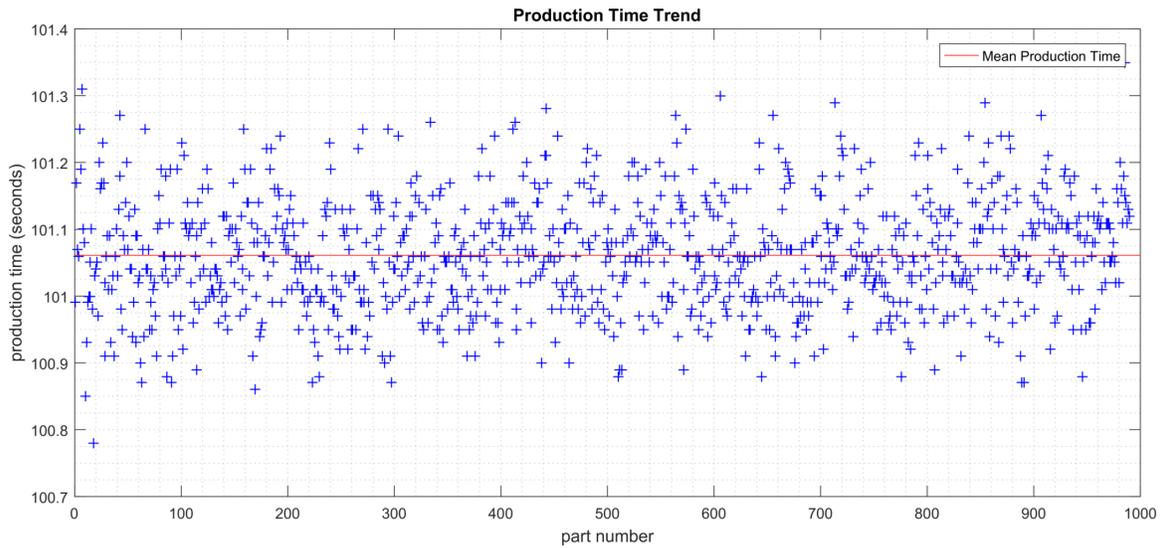
**Fig. 7.** Scatter plot of the part production time KPI from the characterization process data. The horizontal red line denotes the mean part production time.
