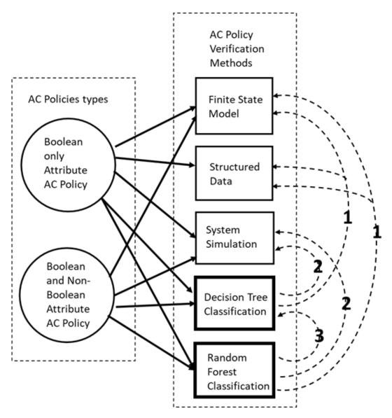
Figure 2: Mapping of access control policy types and verification methods
