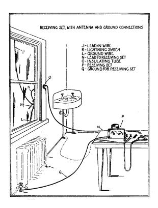
Fig. 2. Diagram showing the antenna and ground connections to the radio.
