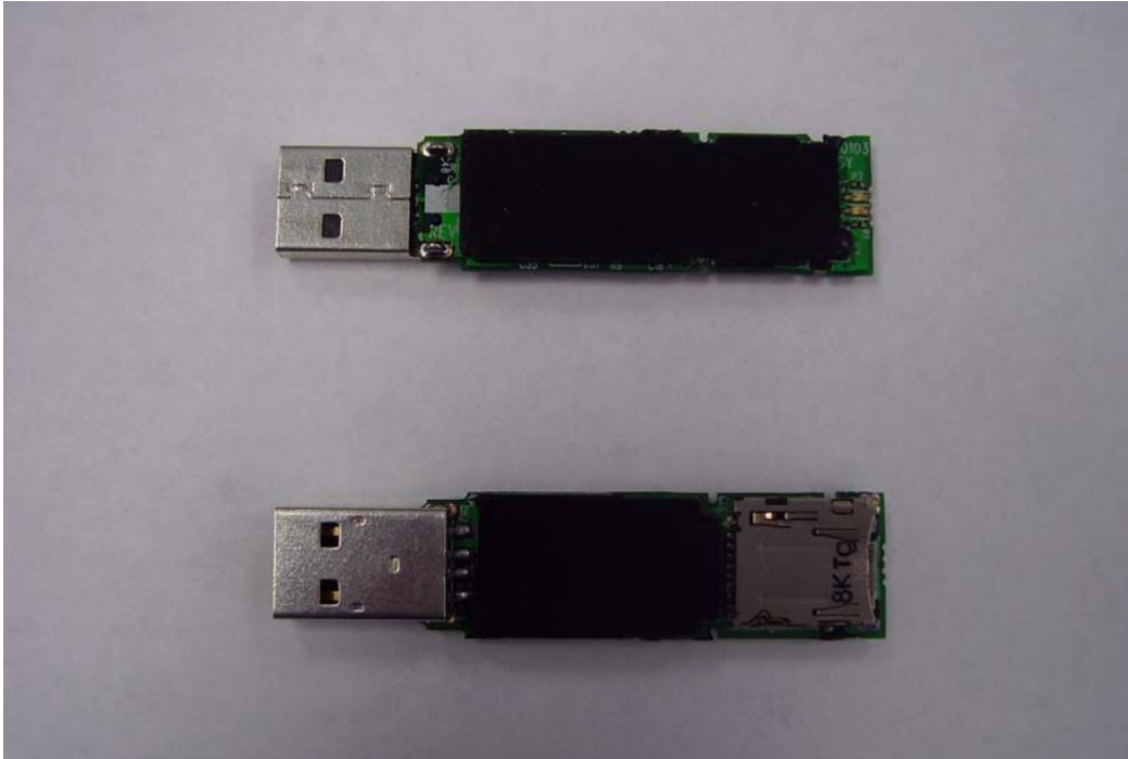
Figure 5: Hydra PC FIPS File Encryption Module without frame extension on PCB (P/N 880070105F) (Top and Bottom Views)
