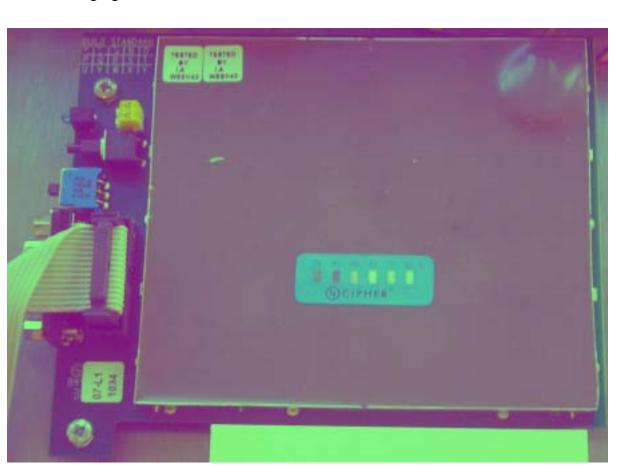
The following figure shows the module mounted inside the NetHSM
