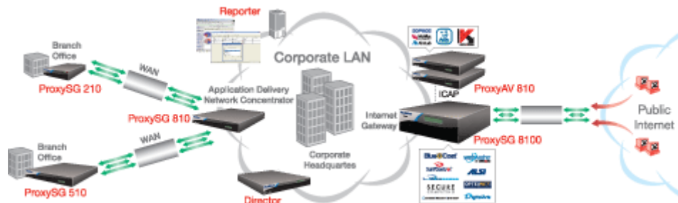
Figure 2 – Typical Deployment of a ProxySG Appliance
