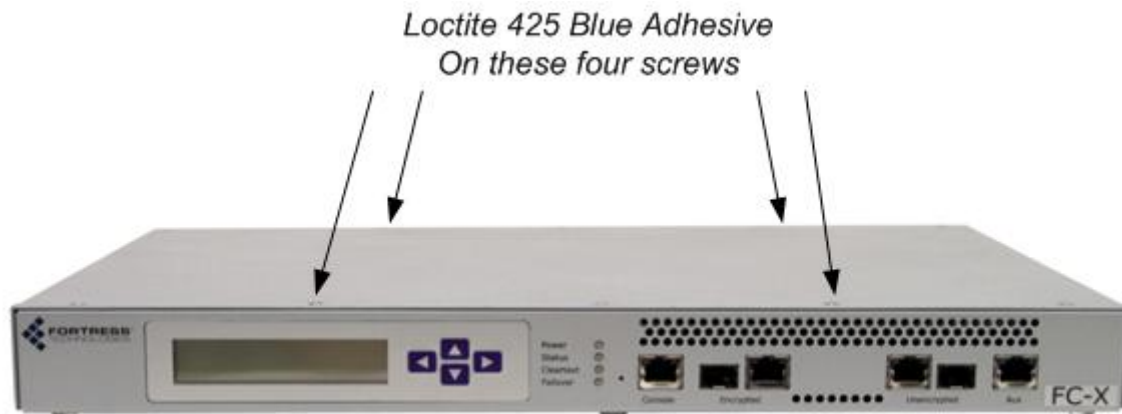
Figure 3: Position of Intrusion Detection Screws
