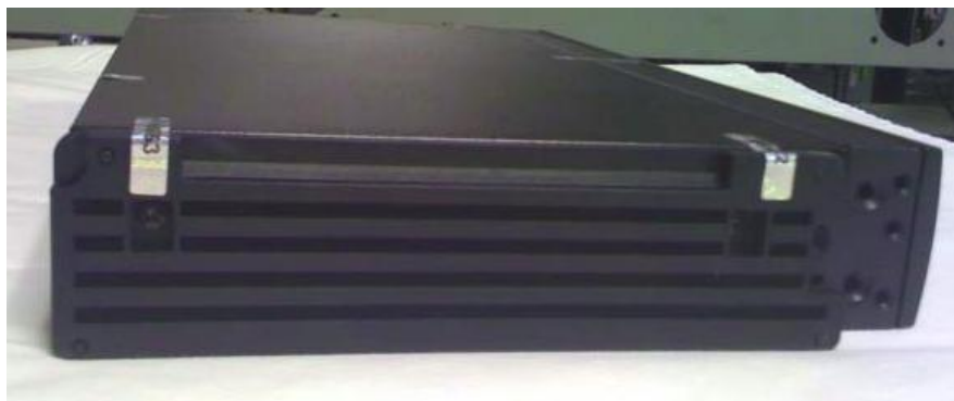
Figure 6 – Tamper-Evident Seal Placement (Left Side View)
