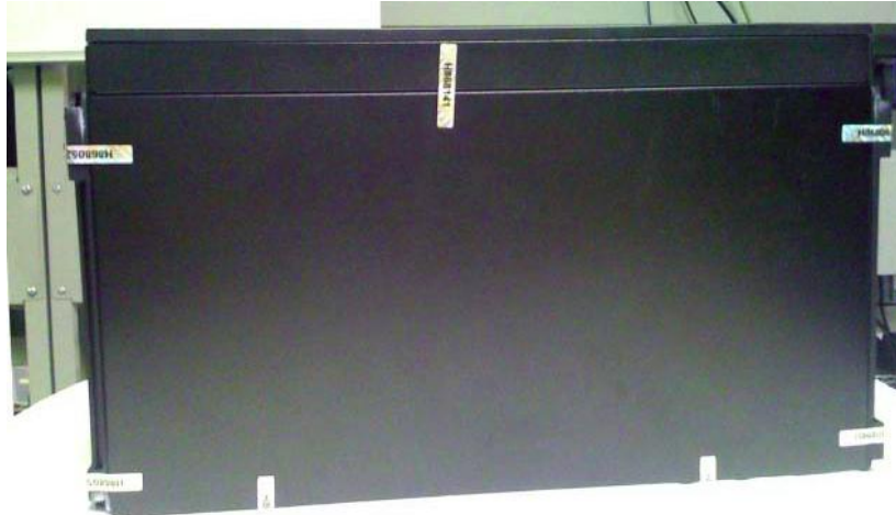
Figure 5 – Tamper-Evident Seal Placement (Top View)
