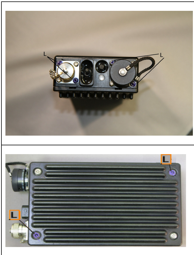
Fig 8.1 ME3 module views with 'loctite' compound over screws and switch mounting (blue color / L label) for tamper evidence and resistance. (views not to scale )
