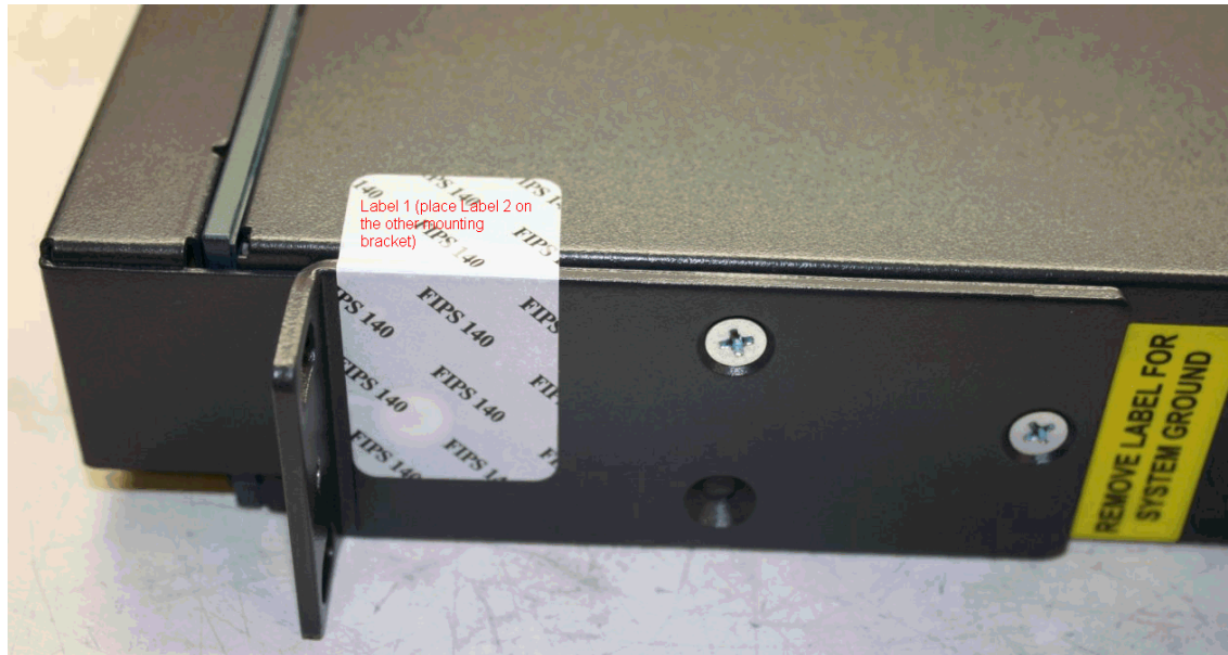
Figure 2 Placement of Tamper-evident Labels on Mounting Brackets
