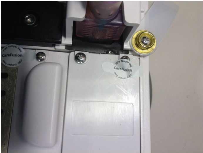
Figure 8-8b: Incorrect application over screw.
