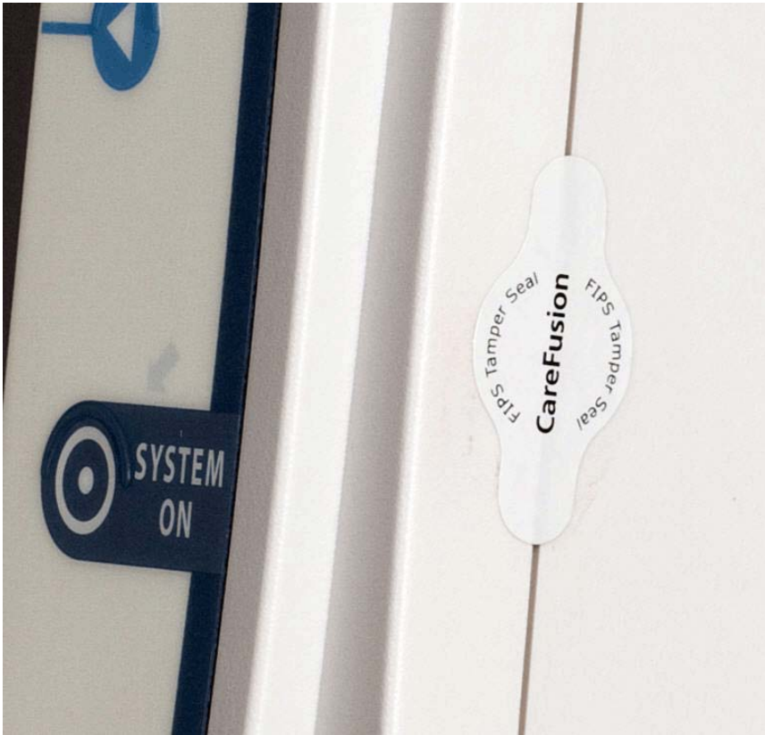
Figure 8-18: Ensure seal is centered between grooves.
