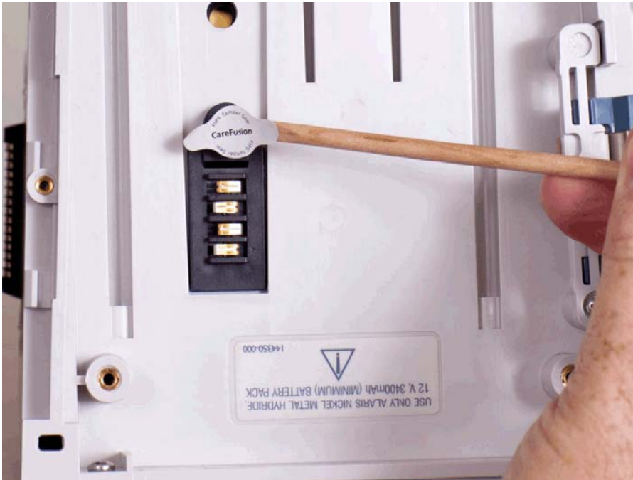
Figure 8-14: Affix seal over battery connector screw.
