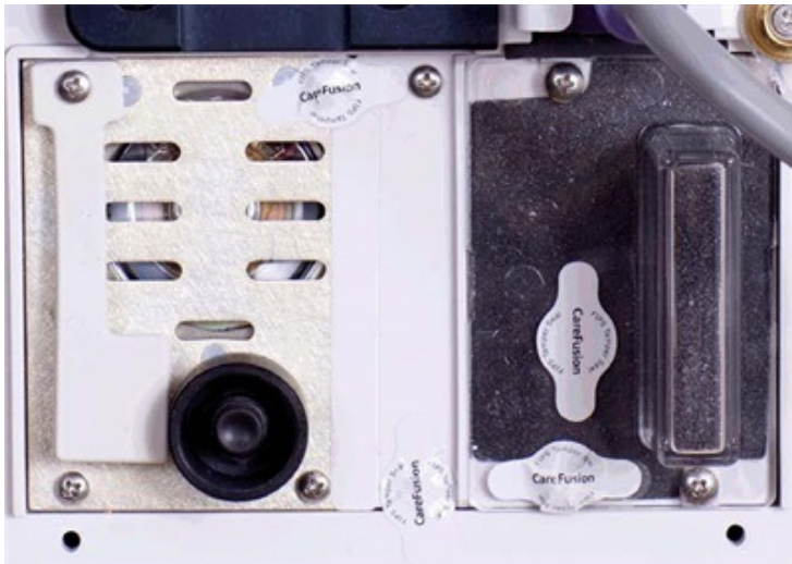
FIGURE 8-2a Back Cover View With Seal Locations: Model 8015 (a/b/g)
