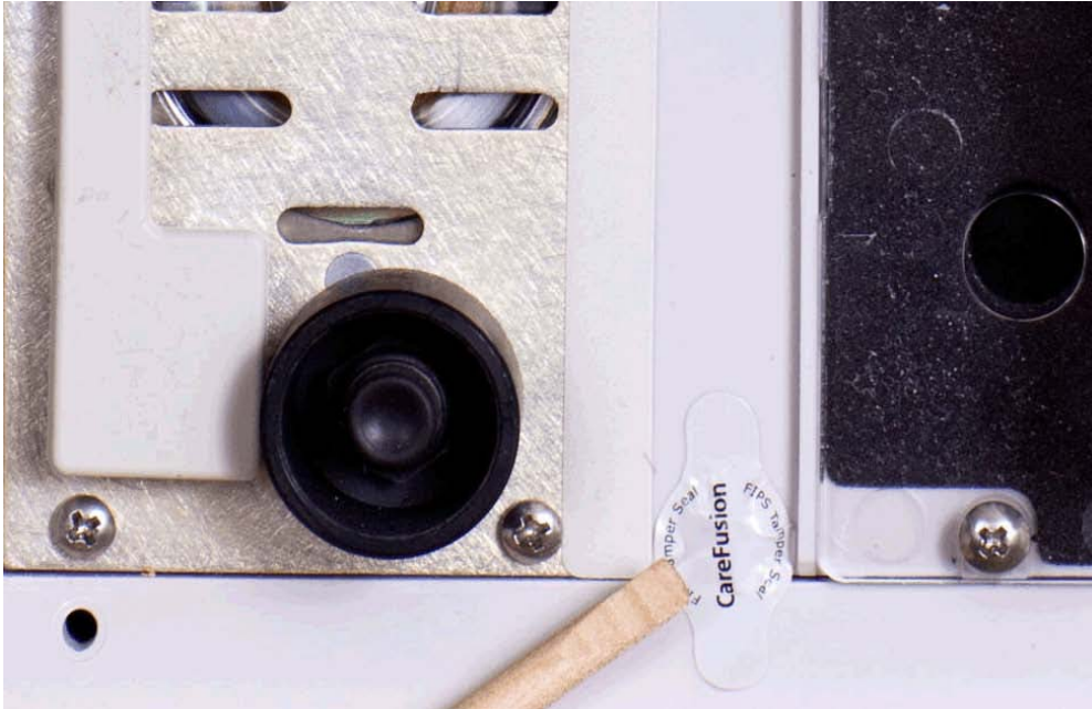
Figure 8-10: Ensure seal covers entire head of screw.
