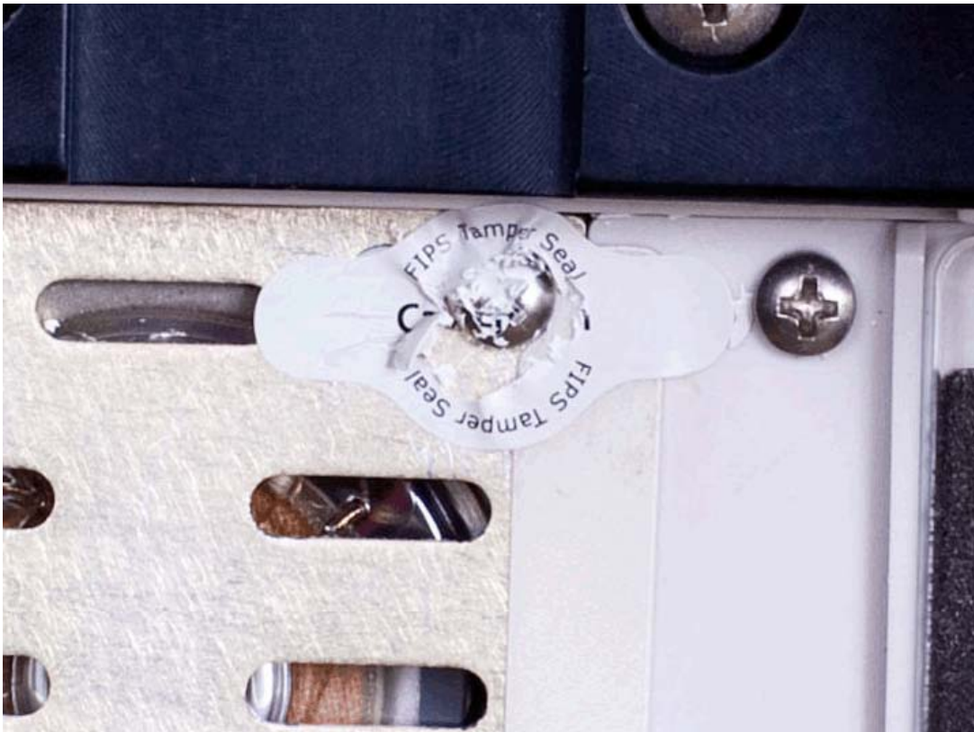
Figure 8-28: Seal has been gouged out.
