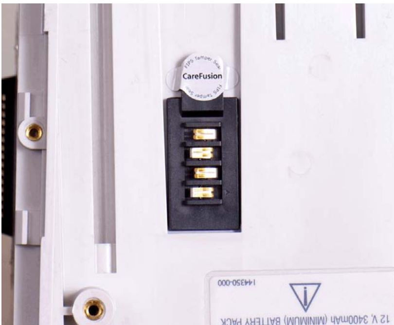
Figure 8-15: Ensure seal covers entire head of screw.
