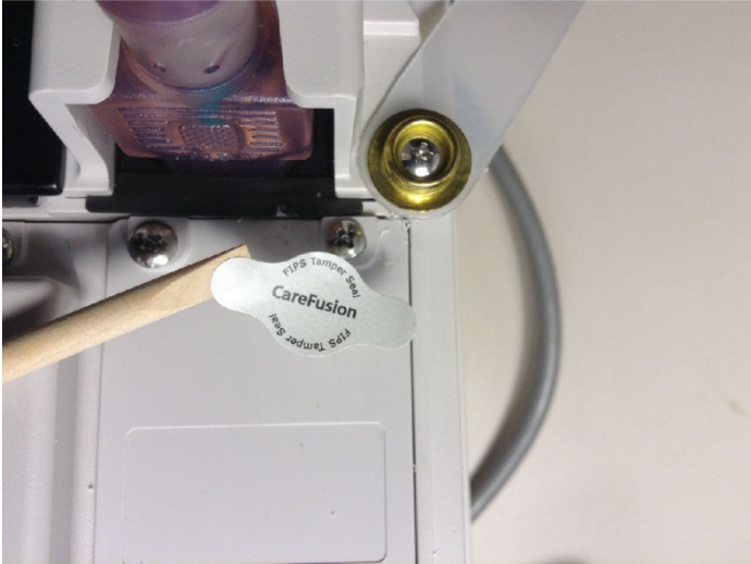
Figure 8-6b: Model 8015 (a/b/g/n) rear panel: Affix seal over the screw in the upper right-hand corner of the rear cover.
