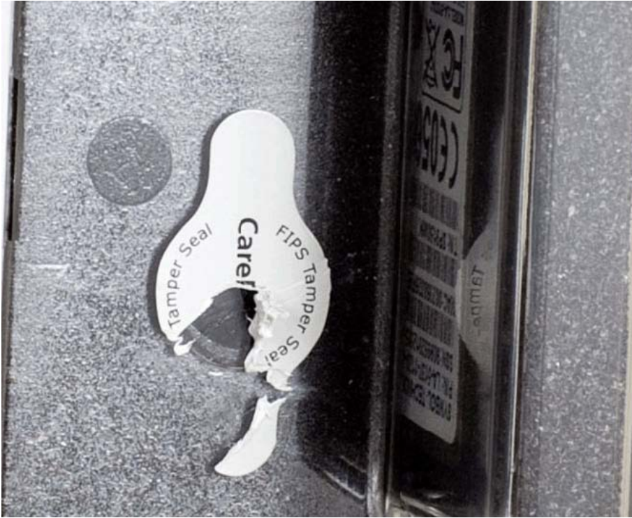
Figure 8-29: Seal has been partially peeled off from the device.
