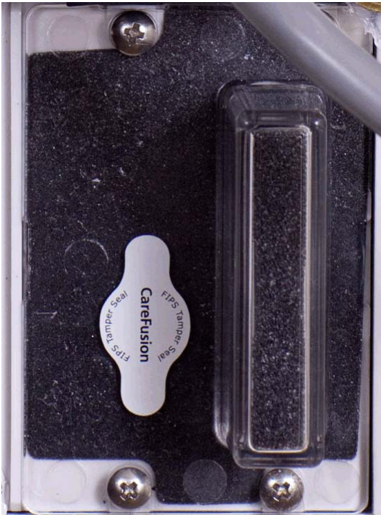
Figure 8-7a: Ensure seal covers entire viewing hole.
