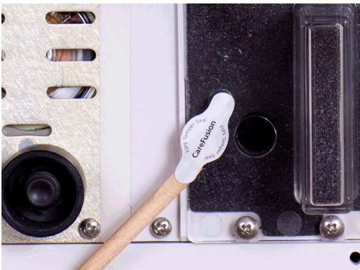
Figure 8-6a: Affix seal over hole in wireless area on Model 8015 (a/b/g) (Note: Rear panel on Model 8015 (a/b/g/n) does not have the hole, see Figure 8-6b).
