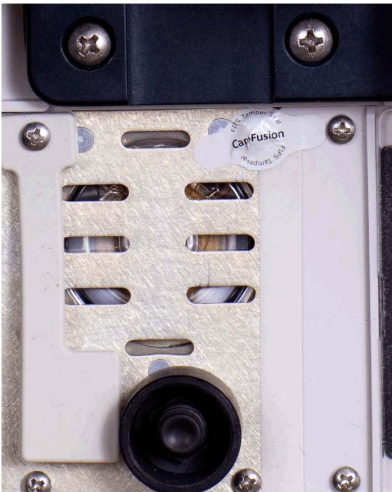
Figure 8-4: Seal must cover entire head of screw.
