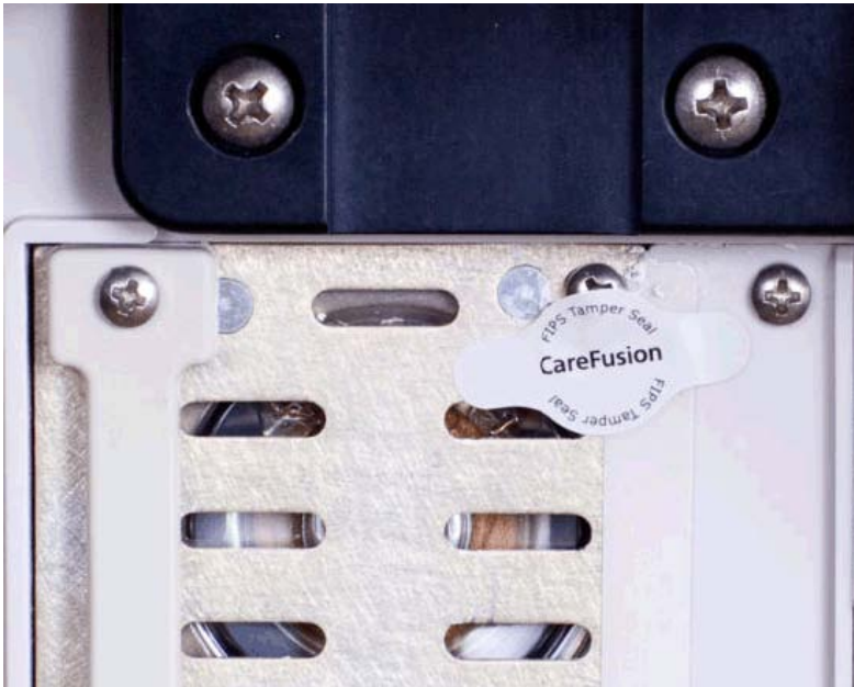
Figure 8-5: Incorrect seal application.
