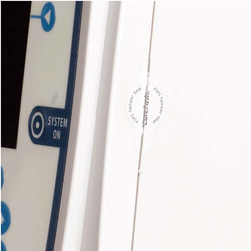
Figure 8-27: Seal has been sliced through.
