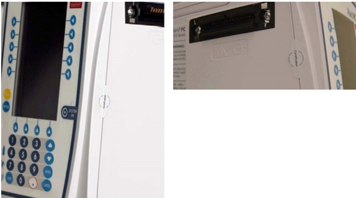
Figure 8-2d: Location of seals over the grooves in the sides of the device.
