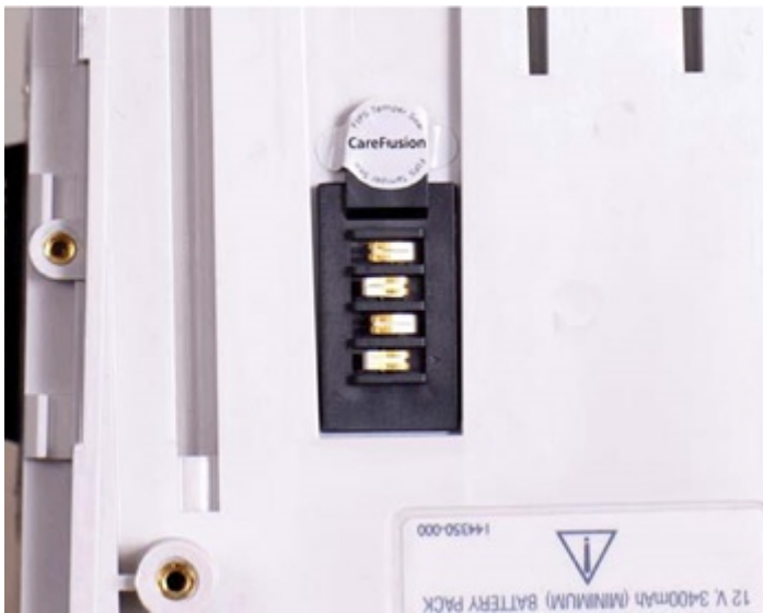
Figure 8-2c: Location of seal on the bottom of the device.
