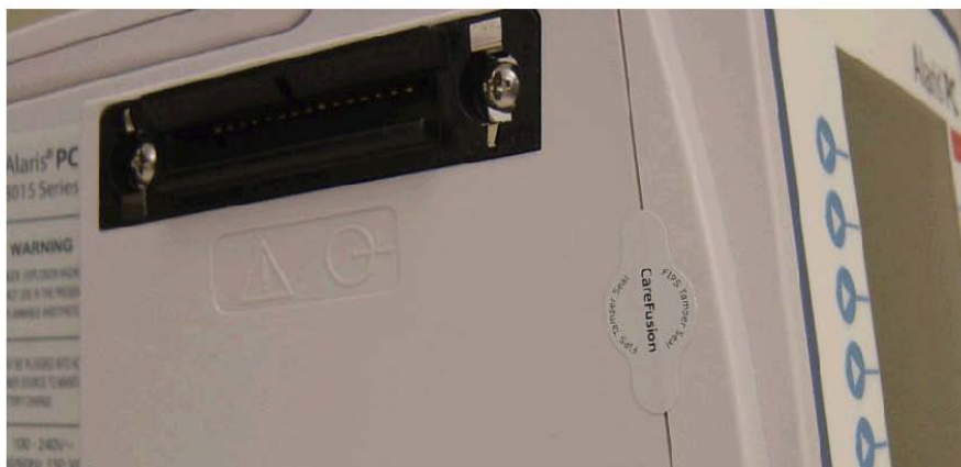
Figure 8-17: Affix a seal on each side of the device.
