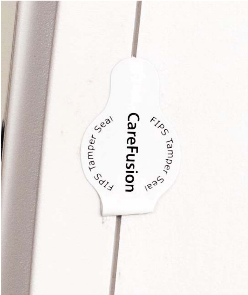
Figure 8-30: Seal has not been applied correctly; not FIPS compliant.
