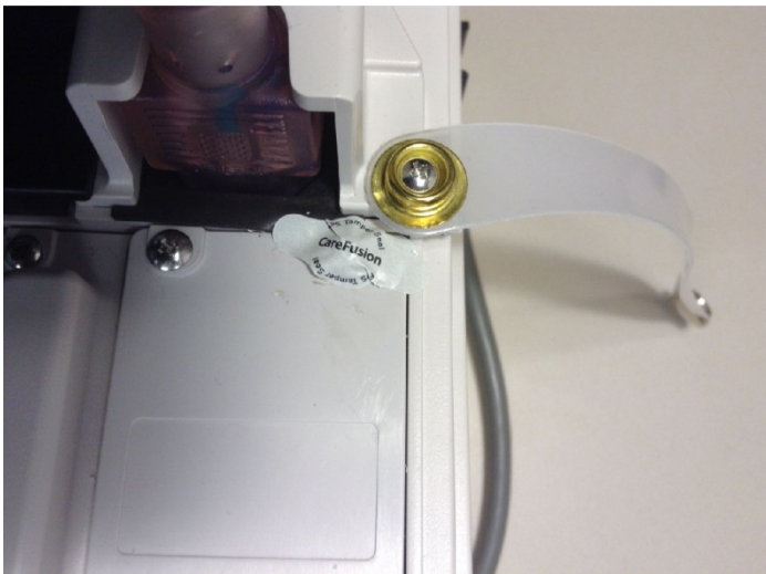
Figure 8-7b: Ensure seal covers entire screw.
