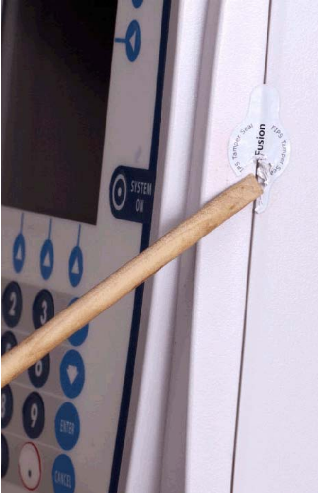
Figure 8-25: Leave no portion of seal remaining.
