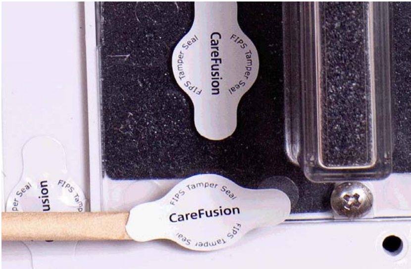
Figure 8-12: Affix seal over bottom screw of wireless card cover.
