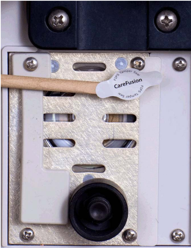
Figure 8-3: Center the seal over middle screw in row beneath black area.
