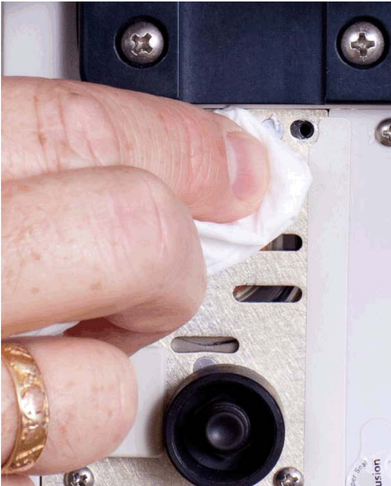
Figure 8-23: Removing remaining debris.
