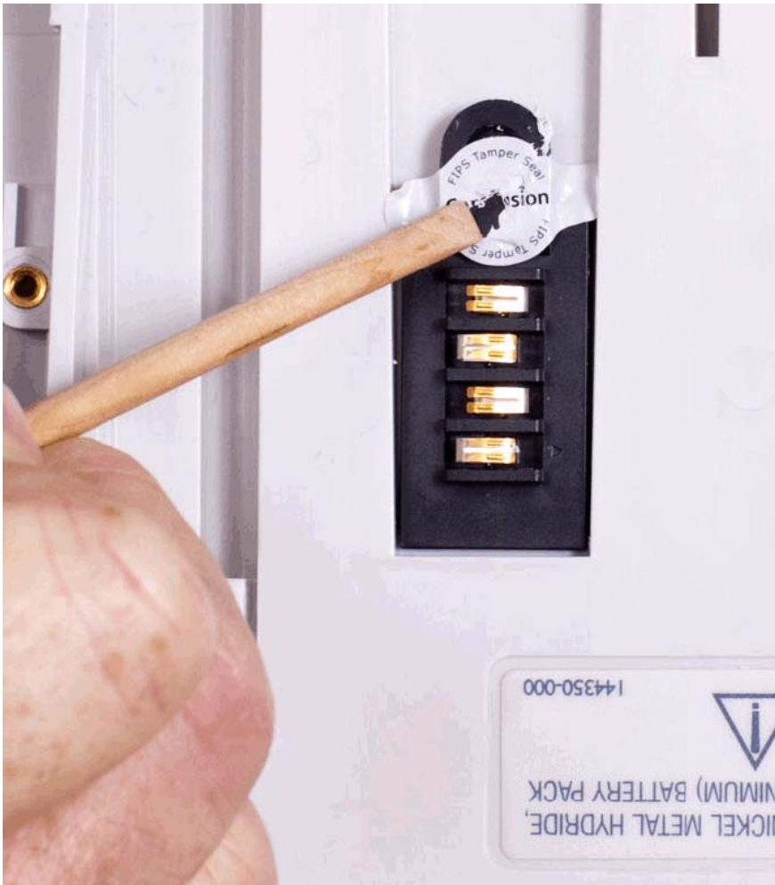
Figure 8-24: Remove seal over battery connector screw.
