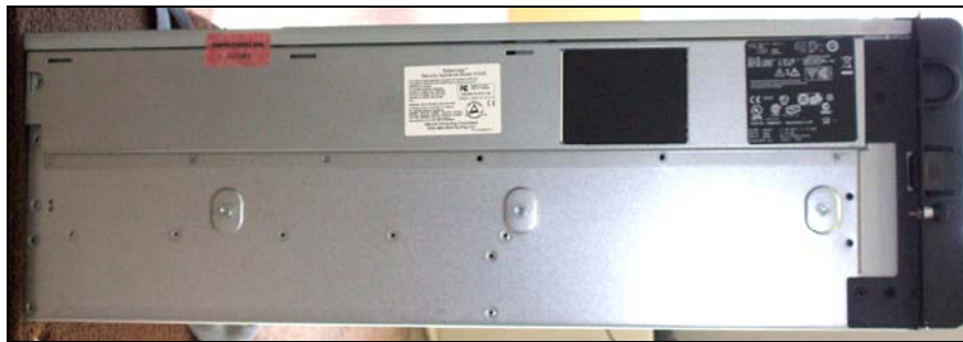
Figure 4 – Tamper-Evident Label Application Instruction Covering the Side Panel
