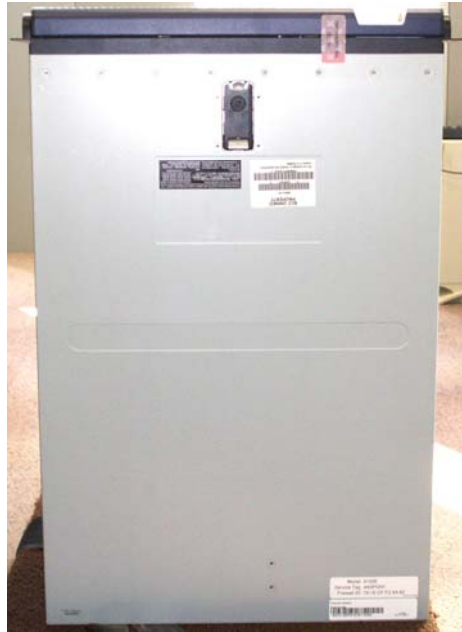
Figure 3 – Tamper-Evident Label Application Instruction Covering the Top and Front Panels
