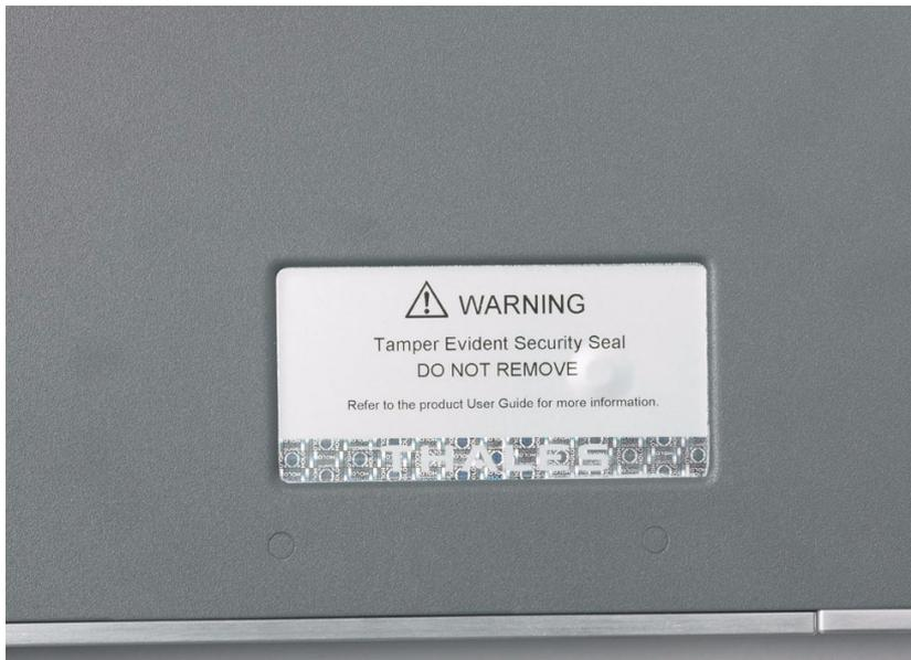
Opening the lid is detected by tamper switches. The lid can only be removed by being slid backwards. There is sufficient overlap between the lid and base that the tamper switches will detect movement at a point where the lid still overlaps the base and before a gap opens that would allow access to circuitry.
