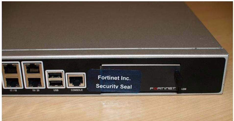
**Figure 15: FortiGate-800 external enclosure seal**
