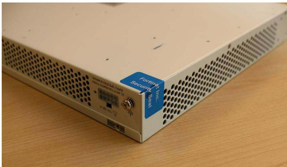
**Figure 9: FortiGate-300A and 300A-HD external enclosure seal**
