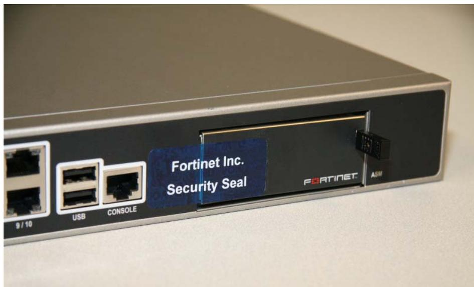
Figure 12: FortiGate-620B external enclosure seal
