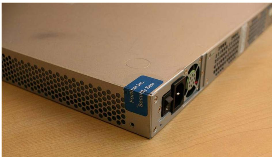
Figure 13: FortiGate-620B external enclosure seal
