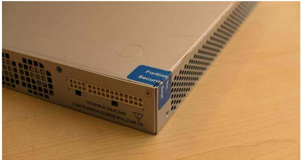
Figure 14: FortiGate-620B AMC faceplate seal
