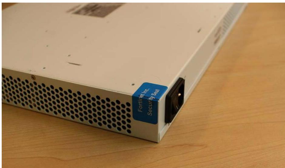
Figure 8: FortiGate-200B external enclosure seal
