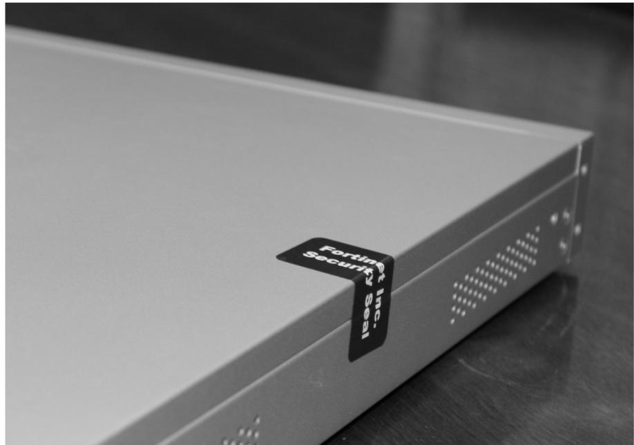
**Figure 10: FortiGate-310B and 311B external enclosure seal**
