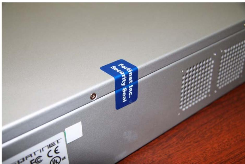
Figure 10: FortiGate-3016B, 3600A and 3810A-E4 power supply seals
