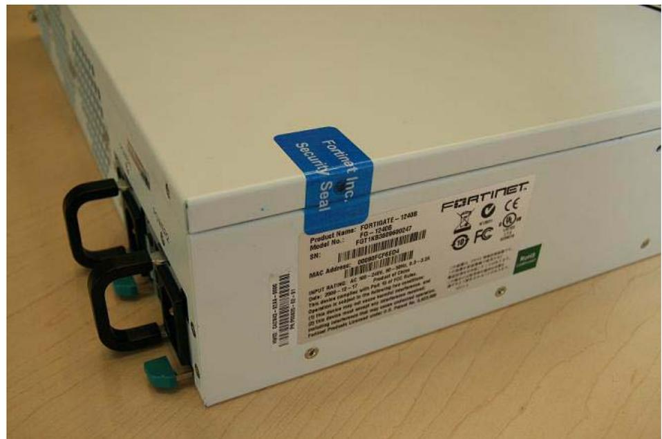
Figure 7: FortiGate-1240B external enclosure seal
