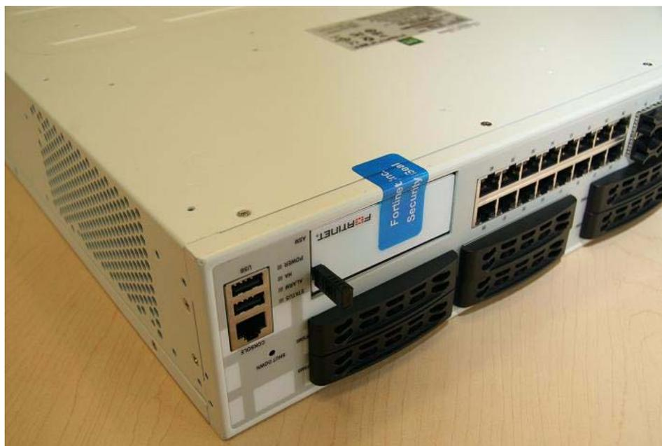
Figure 9: FortiGate-3016B, 3600A and 3810A-E4 external enclosure seal
