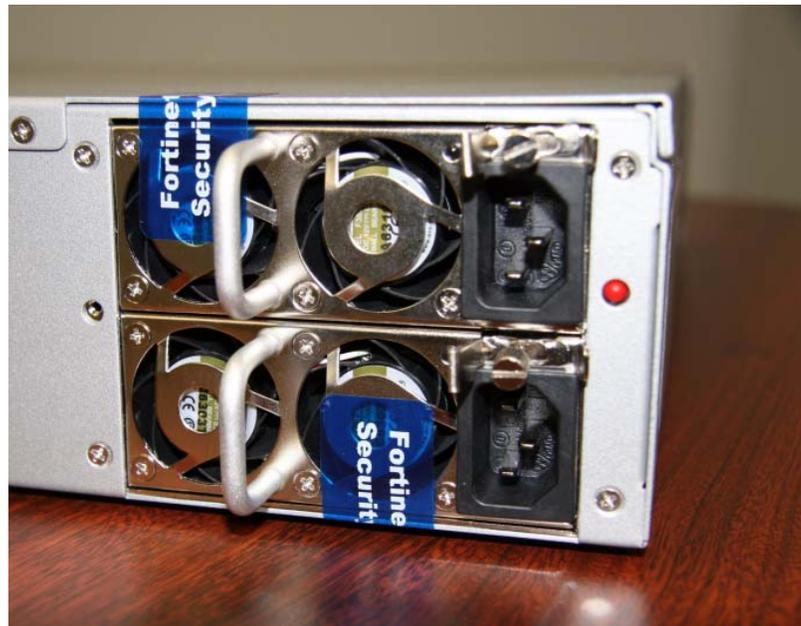
Figure 11: FortiGate-3016B AMC faceplate seal
