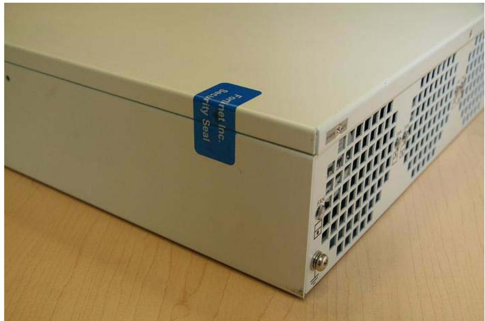
Figure 8: FortiGate-1240B AMC faceplate seal
