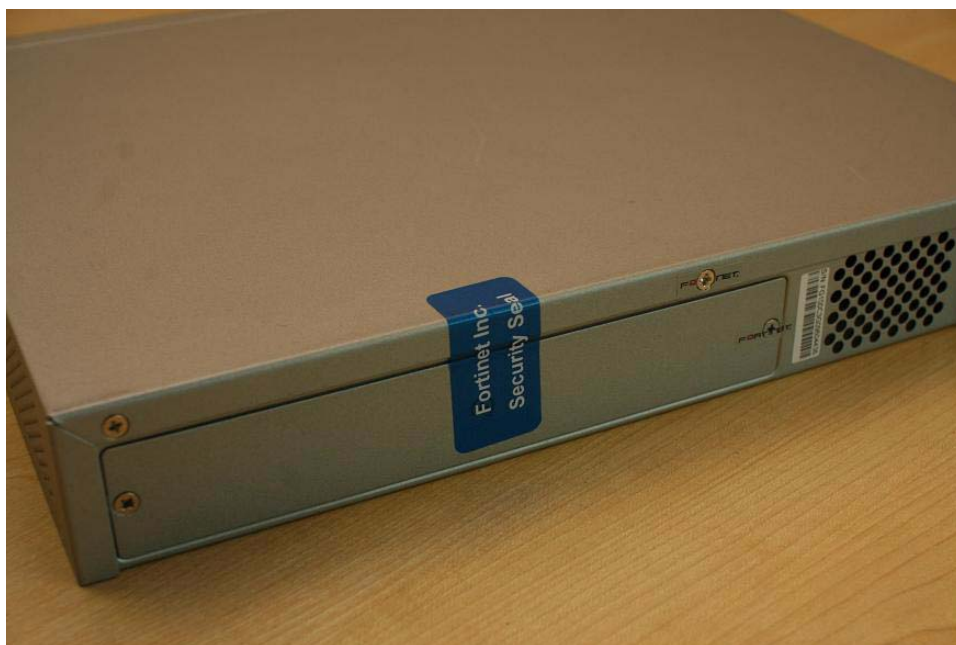
Figure 9: FortiGate-110C cover plate seal
