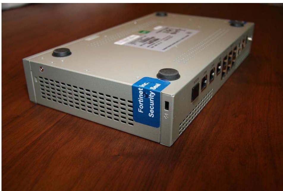
Figure 5: FortiGate-80C external enclosure seal
