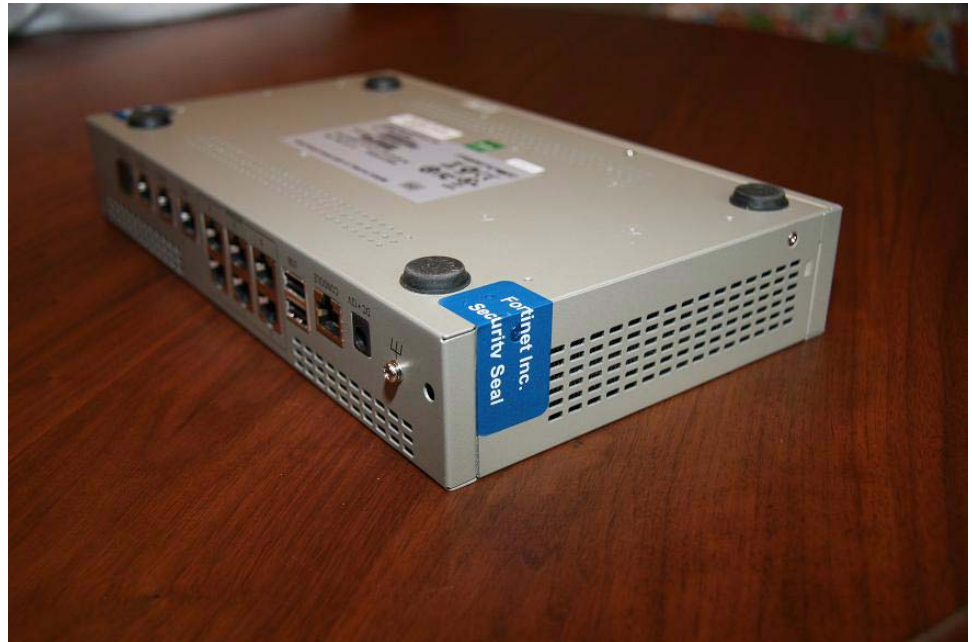
Figure 6: FortiGate-80C external enclosure seal
