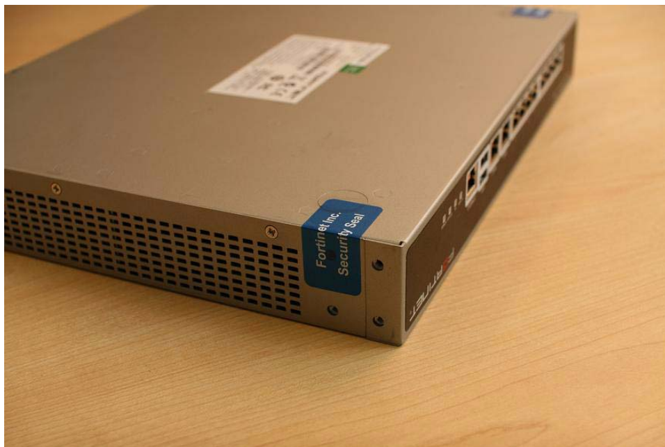
Figure 8: FortiGate-110C and 111C external enclosure seal
