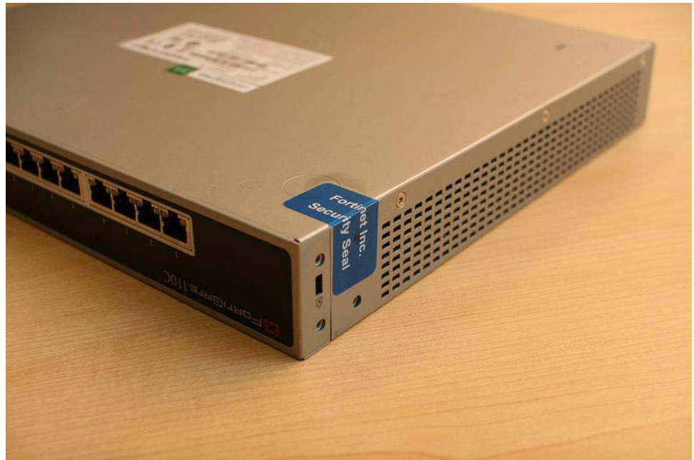
Figure 7: FortiGate-110C and 111C external enclosure seal
