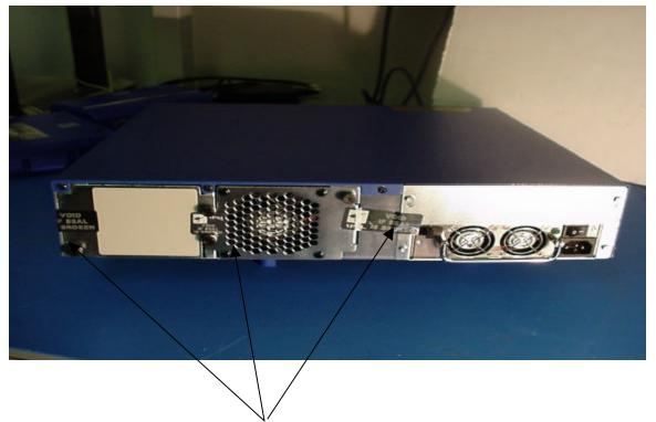
Install one small tamper proof label 74-0104 (middle) and two tamper proof labels 74-0069 to the rear of VSU-5000 system as shown.
