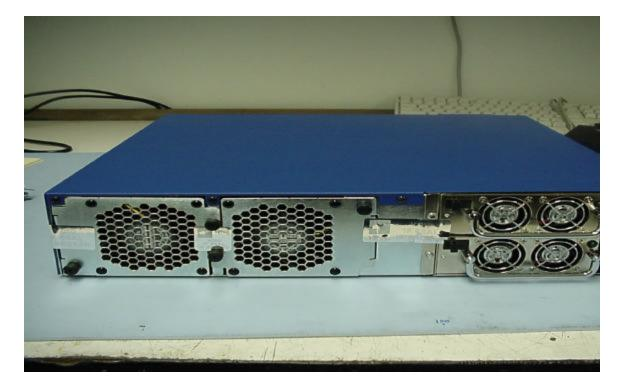
Install one small tamper proof label 74-0104 (middle) and two tamper proof labels 74-0069 to the rear of VSU-7500 system as shown.
