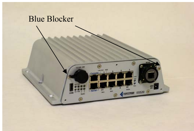
Figure 5: ES520 Version 2 Tamper Evidence
