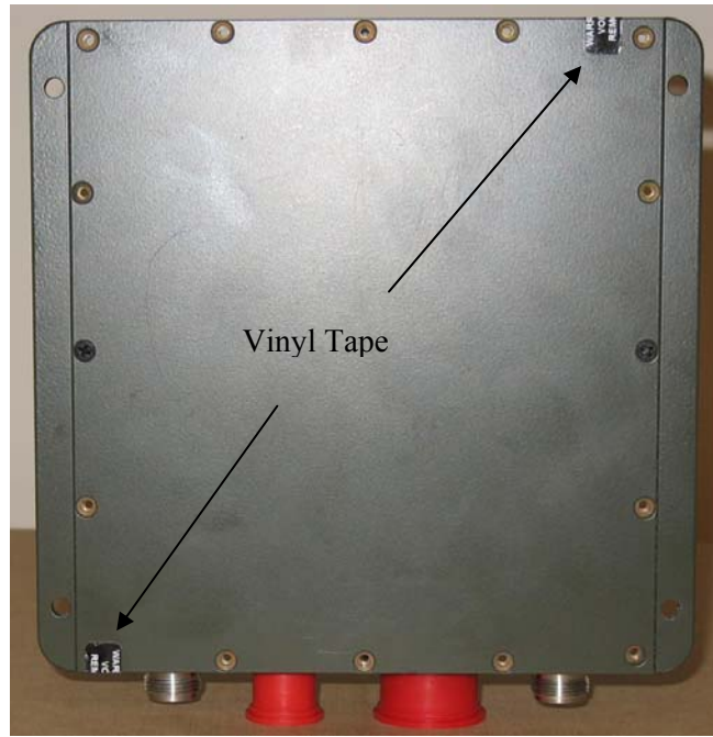
Figure 6: ES820 Tamper Evidence
