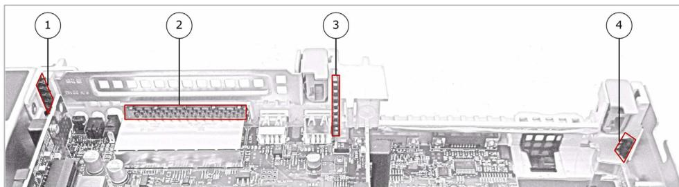
**Figure 7 – Velcro Strip Placement in Rear of Chassis**
