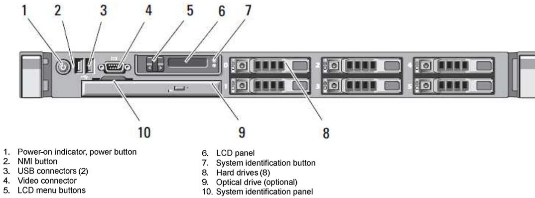
**Figure 3 – Front Panel Features and Indicators**
