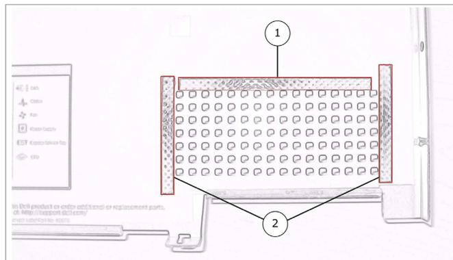
**Figure 6 – Velcro Strip Placement on Top Cover**
