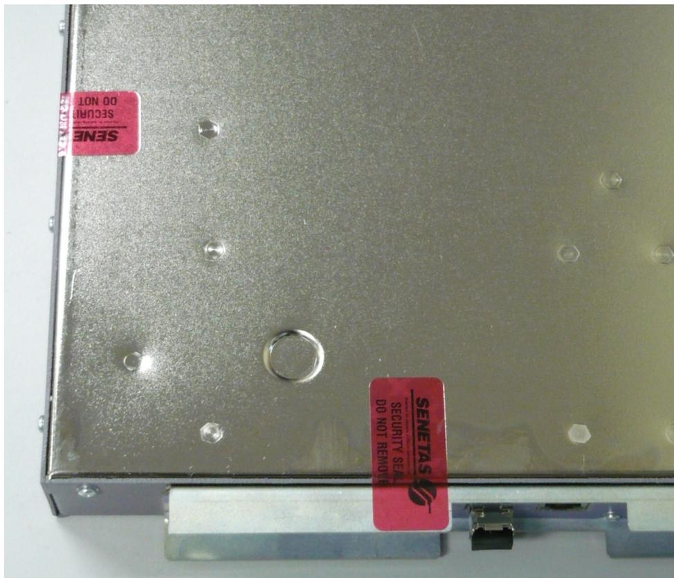
**Figure 7 – Factory installed tamper seals**
