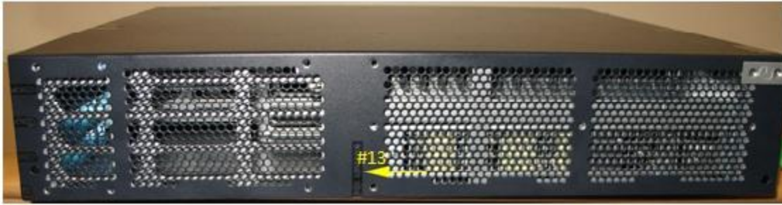
Figure 3. SRX650 Tamper Evident Seal Location (Right Side)
