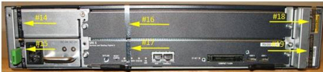
Figure 4. SRX650 Tamper Evident Seal Location (Rear)
