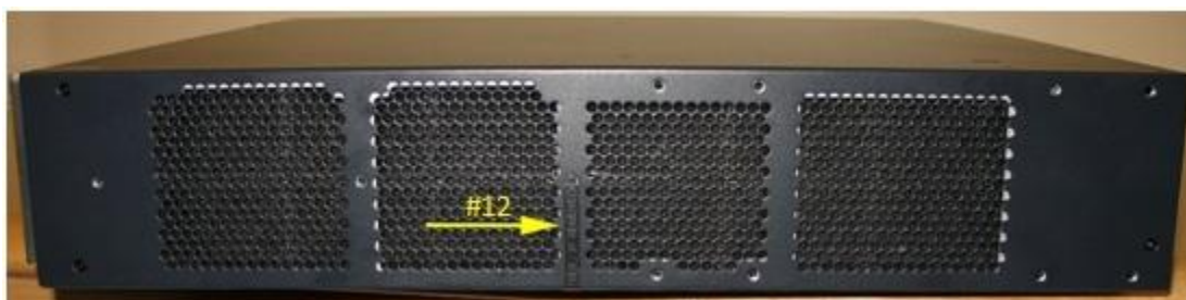
Figure 2. SRX650 Tamper Evident Seal Location (Left Side)
