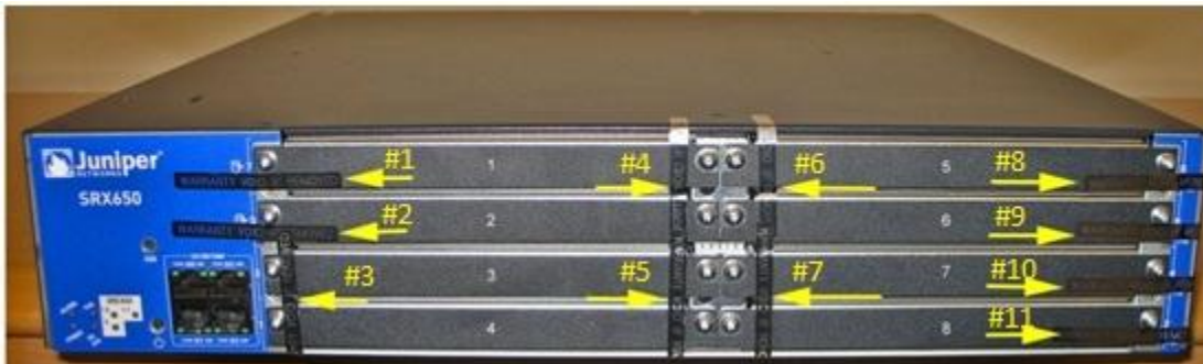
Figure 1. SRX650 Tamper Evident Seal Locations (Front)
