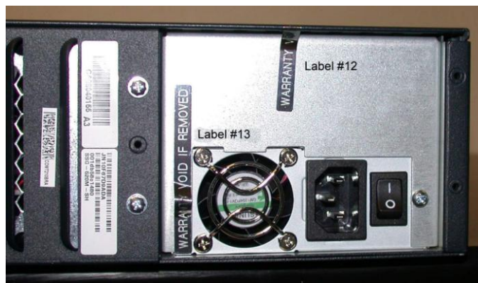
Figure 4: Rear detail of the SSG 520M
