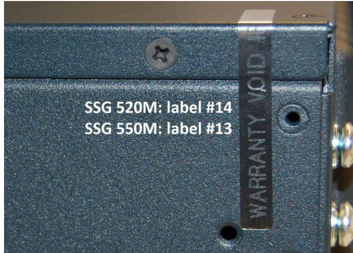
Figure 6: Rear corner of the SSG 520M and 550M
