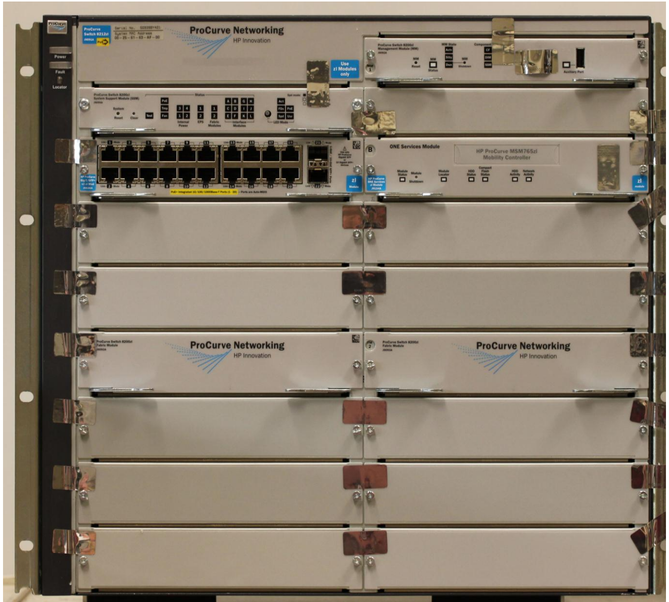
Figure 4 shows the front of the HP 8212 zl Switch with the HP MSM765zl Mobility Controller.
