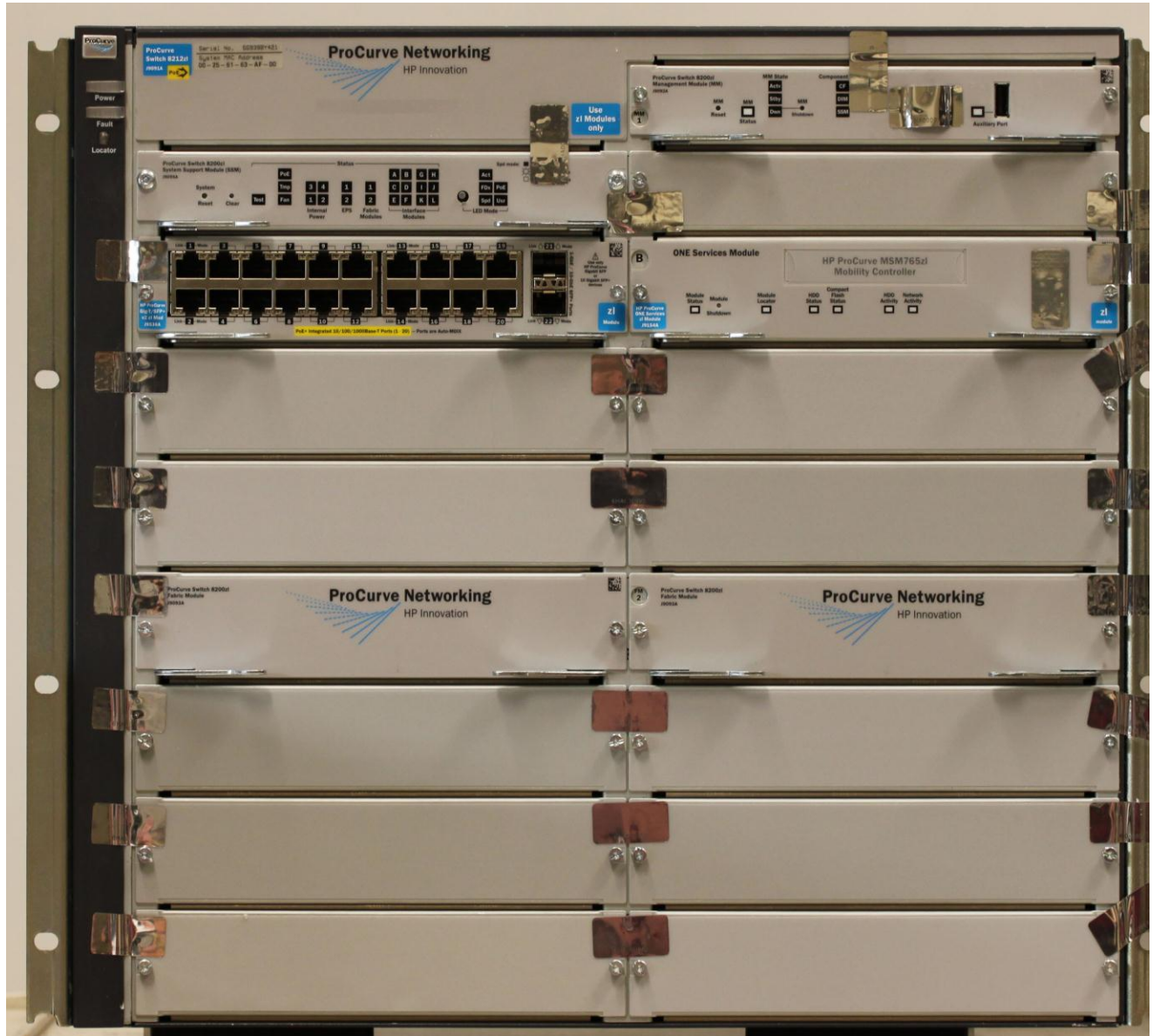
Figure 4 – HP 8212 zl Switch with the HP MSM765zl Mobility Controller
