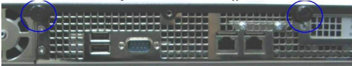
**Figure 9 Rear Baffle Screw Removal**
