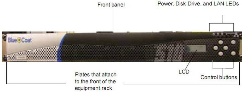
**Figure 4 Front View of the ProxySG 510**
