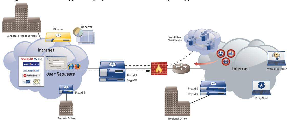
**Figure 1 Typical Deployment of a ProxySG Appliance**
