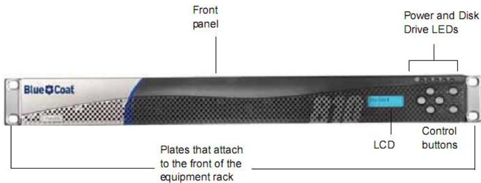
**Figure 5 Front View of the ProxySG 810**
