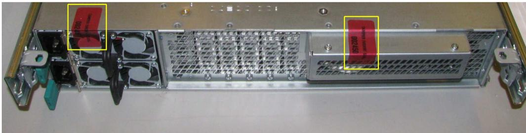
**Figure 19 – Tamper-Evident Seal Application Positions (S5032/S6032 – Bottom Rear)**
