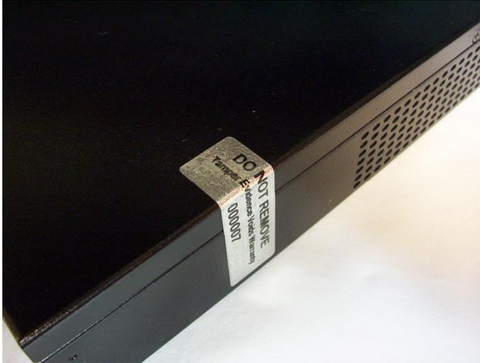
At the factory the serialized tamper evident seal shall be applied as follows::
