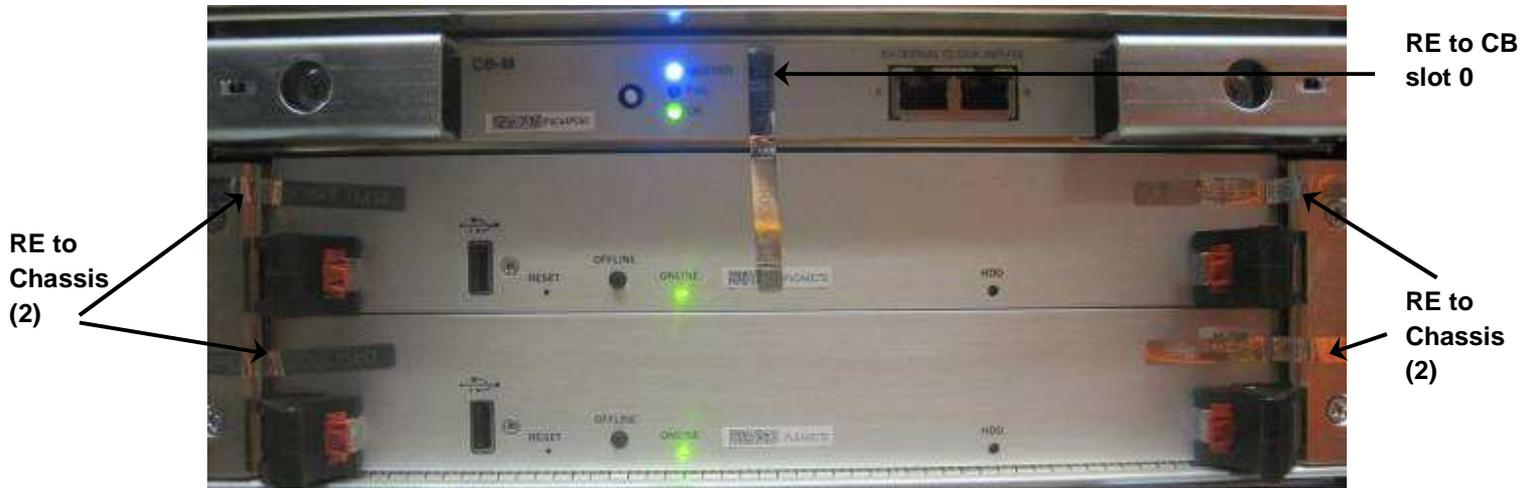
The M320 houses the RE-A-2000-4096. The physical boundary is the M320 chassis containing two routing engine units mounted next to a control board and sealed in place with five (5) tamper evident labels. The label placement for the physical boundary is identified in the figure above. Note that the additional slots of the M320 chassis are not part of the physical boundary, and the boundary traces the two routing engine units mounted next to a control board and the inside of the M320 chassis.
