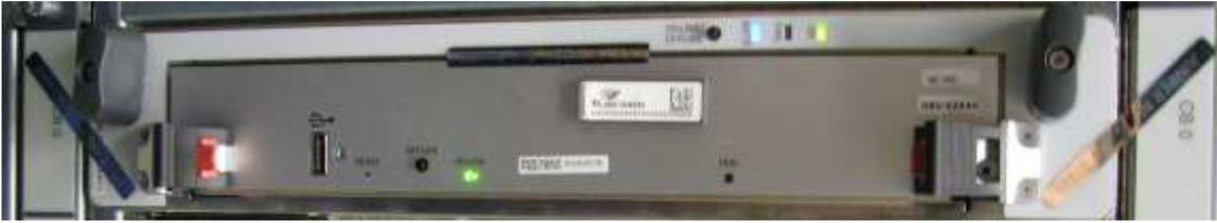
Figure 4A. M120 FIPS Physical Boundary - M120 Chassis and Routing Engine RE-A-2000 is slots marked as RE0 and RE1
