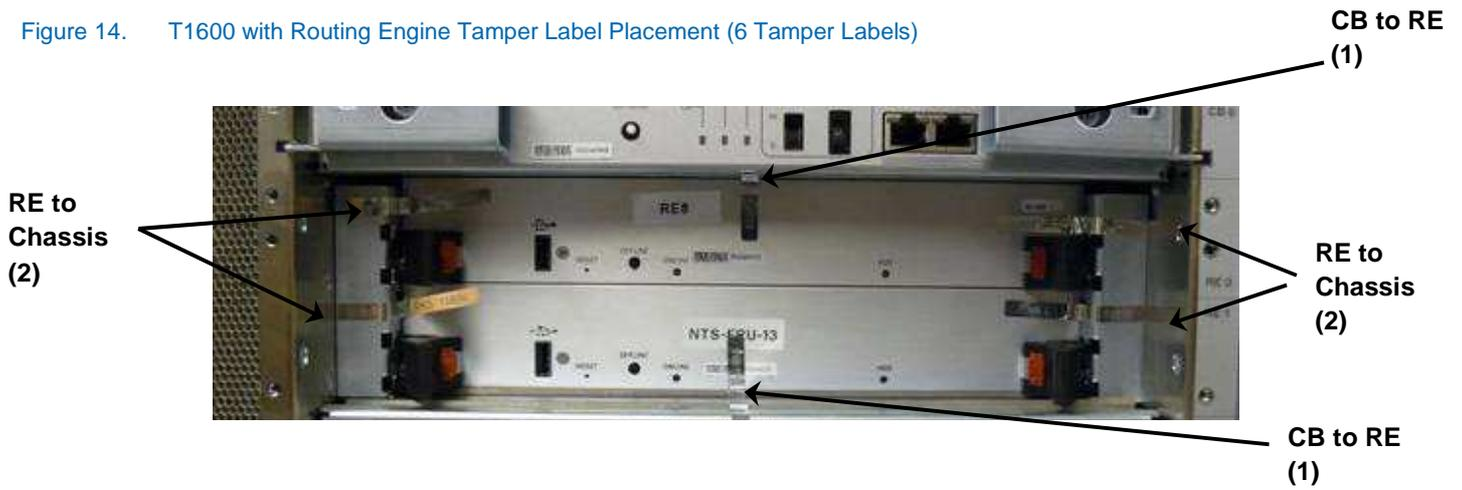
Figure 15. Alternate View - T1600 with Routing Engine Tamper Label Corner Placement for CB to RE
