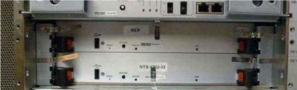
Figure 9A. T1600 FIPS Physical Boundary- T1600 Chassis RE-A-2000 in slots marked as RE1 and RE0, and Control Board in slot marked as CB0
