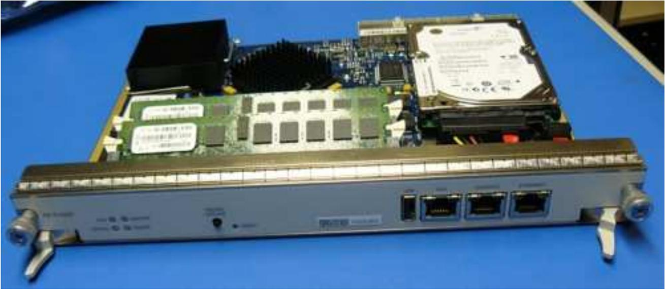
Figure 4. M120 with Routing Engine
