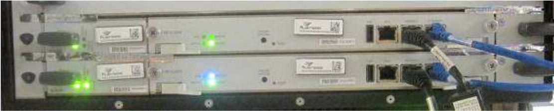
Figure 8A. MX960 Physical Boundary- MX960 Chassis, RE-S-2000 in RE housing, in slots marked as 6 and 7, and a blanking plate in slot 8.
