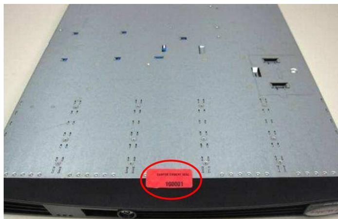
**Figure 12 – C2050/C3000 Tamper-Evident Seal Placement (Bottom)**
