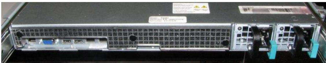
**Figure 15 – C2050 Security Baffle Placement**
