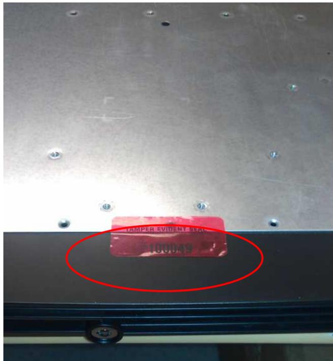
**Figure 10 – CI015 Tamper-Evident Seal Placement (Bottom)**
