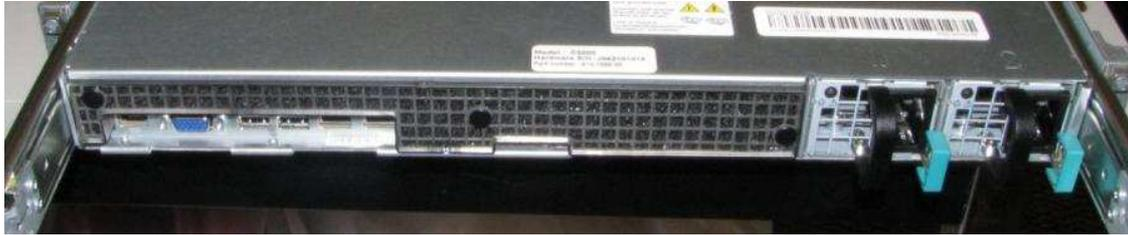
**Figure 16 – C3000 Security Baffle Placement**
