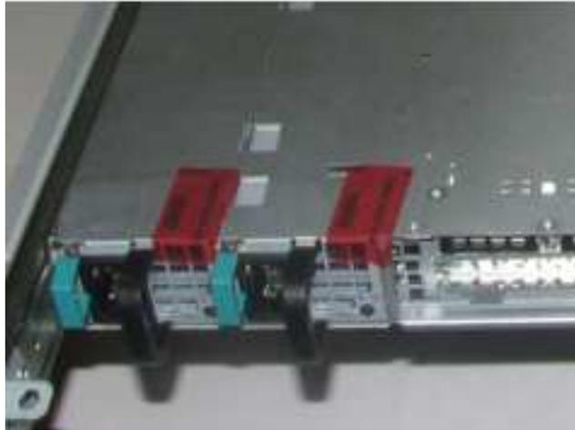
**Figure 13 – C2050/C3000 Power Supply Tamper-Evident Seal Placement (Bottom)**
