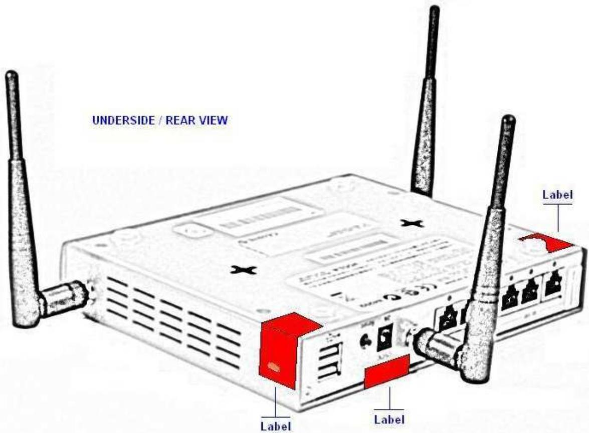
Figure 18: WatchGuard XTM 2 Series Tamper Evident Label Placement
