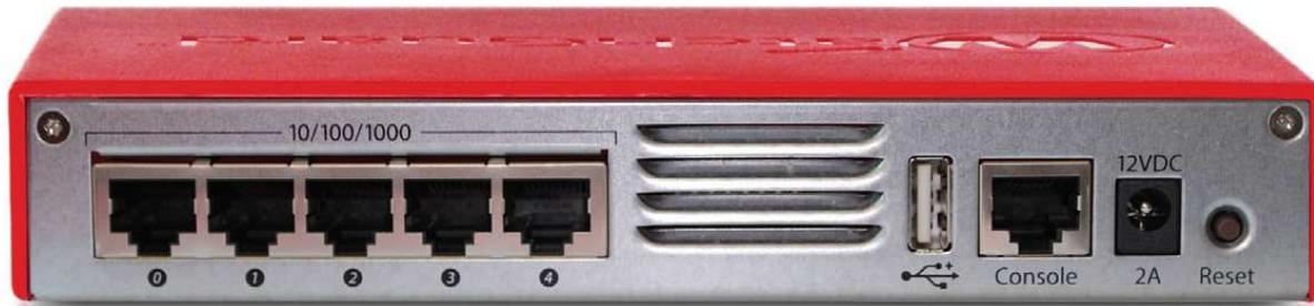
Figure 4: XTM 25 and XTM 26 Rear View
