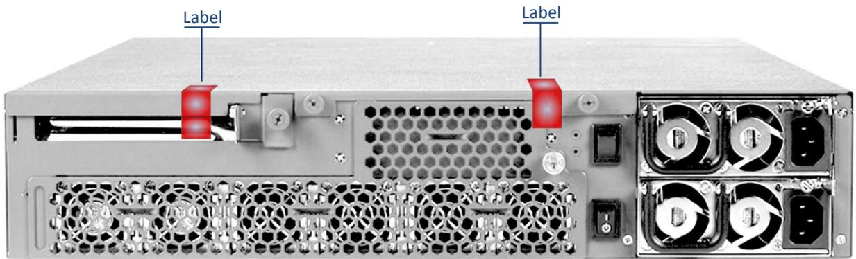
Figure 25: WatchGuard XTM 2050 Tamper Evident Label Placement
