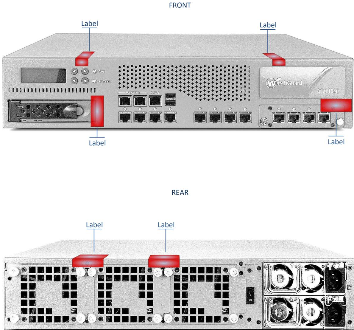
**Figure 24: WatchGuard XTM 1050 Tamper Evident Label Placement**
