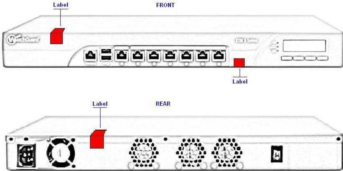
Figure 22: WatchGuard XTM 5 Series Tamper Evident Label Placement
