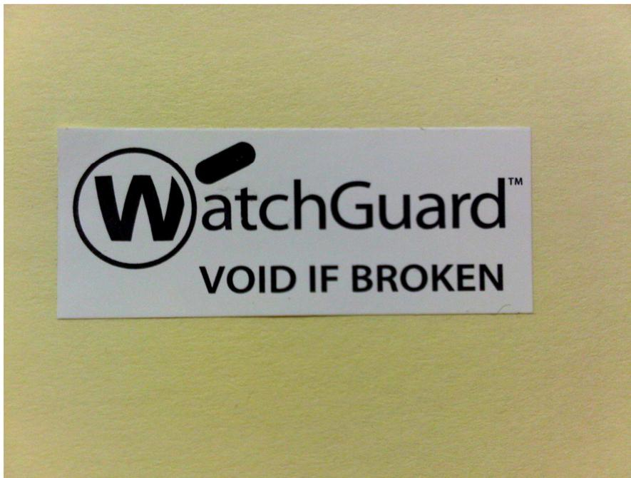
**Figure 17: WatchGuard XTM Tamper Evident Label**
