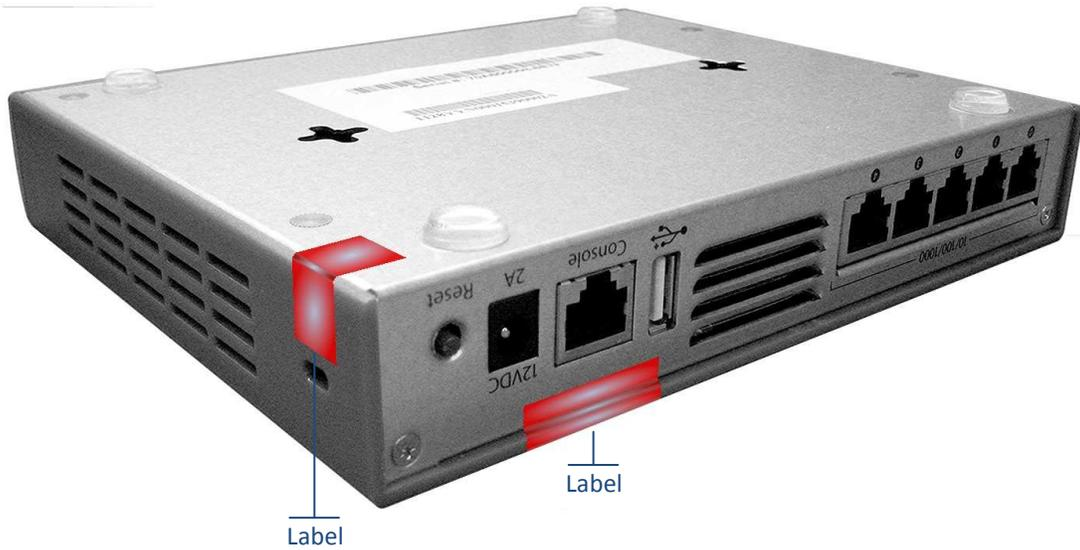
Figure 19: WatchGuard XTM 25/26/33 Tamper Evident Label Placement
