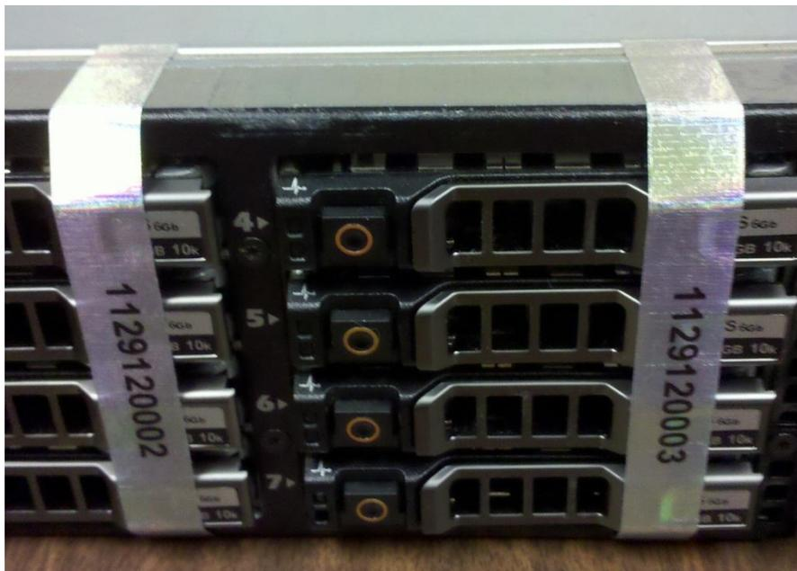
**Figure 18: G10 Labels on Hard Drive Bays**
