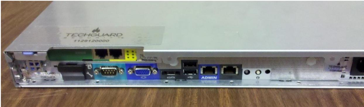
**Figure 13: G01 Rear Opacity Shield and Labels for RJ45 Model**
