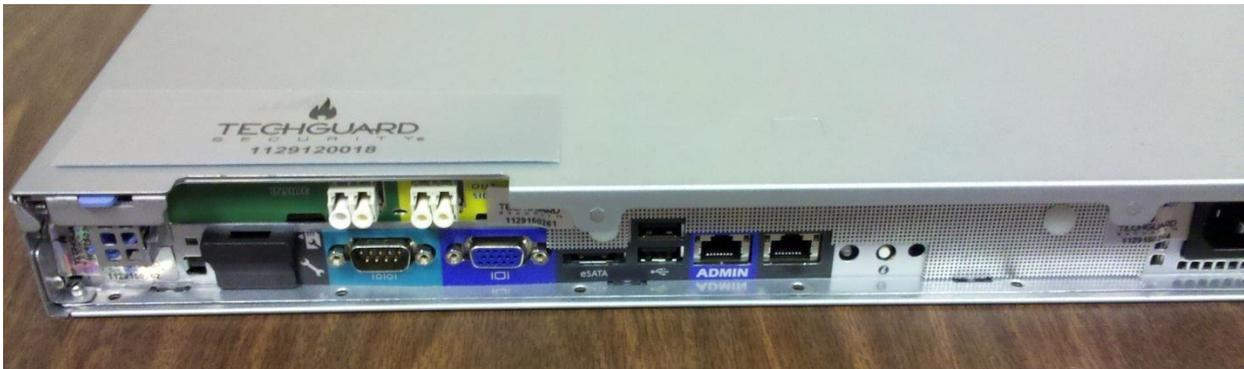
**Figure 14: G01 Rear Opacity Shield and Labels for Fiber Model**
