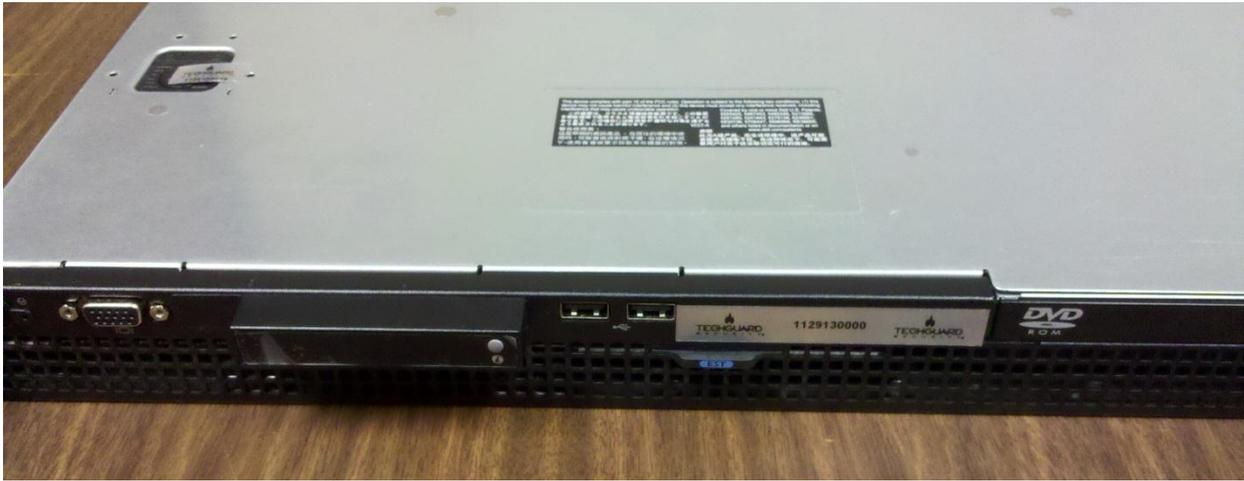
**Figure 12: G01 Front and Lock Tamper Evident Labels**
