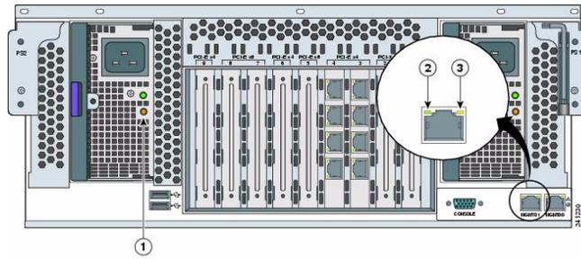
Figure 8 – Cisco ASA 5580 Series Security Appliance Rear Panel Indicators
