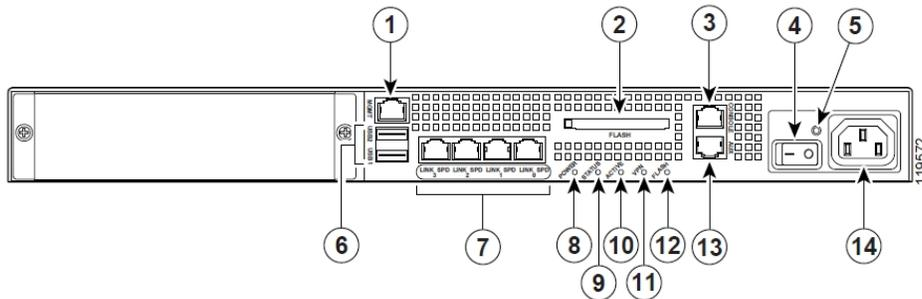
Figure 5a – Cisco ASA 5510, 5520, 5540 Series Security Appliance Rear Panel
