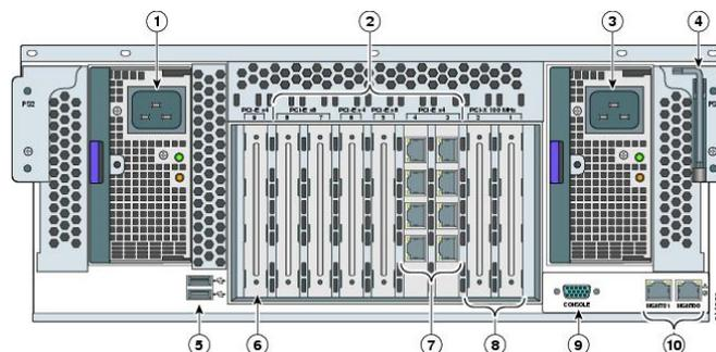
Figure 9 – Cisco ASA 5580 Series Security Appliance Rear Panel
