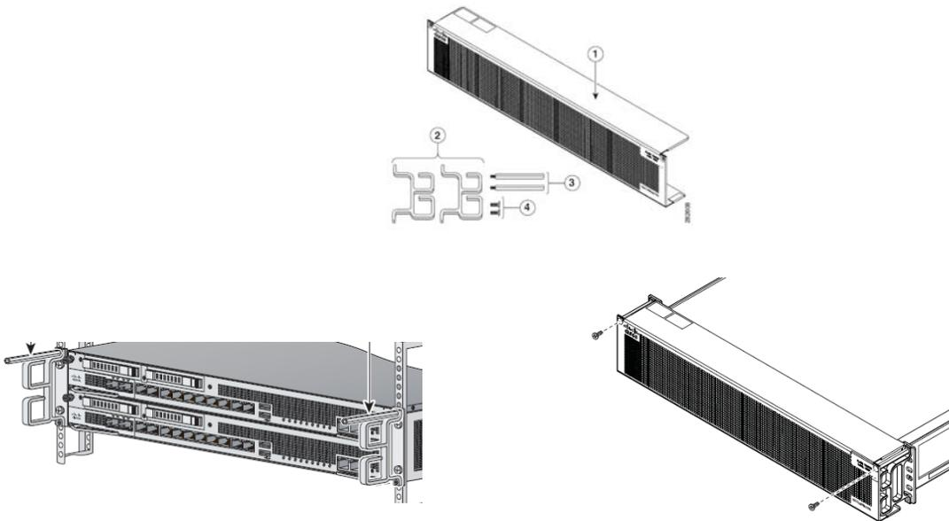
**Figure 18 – ASA 5585-X Front Opacity Shield Placement**
