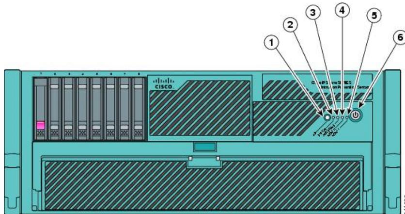
Figure 7 – Cisco ASA 5580 Series Security Appliance Front Panel
