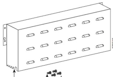
**Figure 17 – ASA 5580 Rear Opacity Shield Placement**
