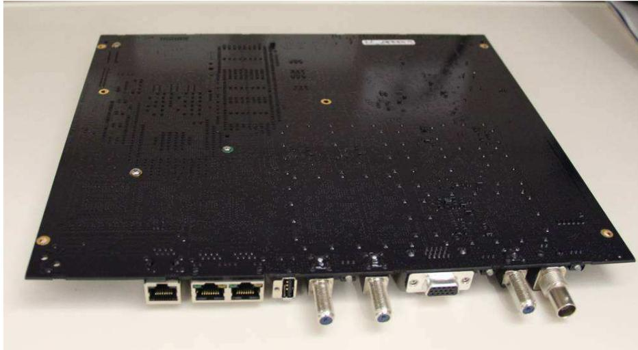
**Figure 3 – iConnex e800-FIPSL2 Satellite Router Board (Bottom)**
