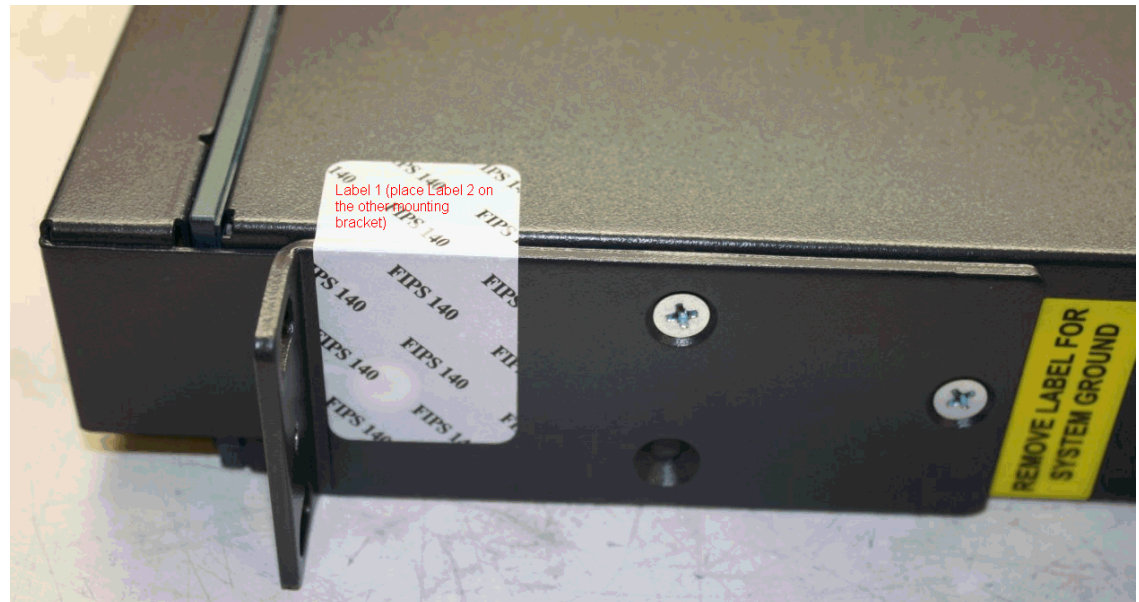
Figure 2 Placement of Tamper-evident Labels on Mounting Brackets
