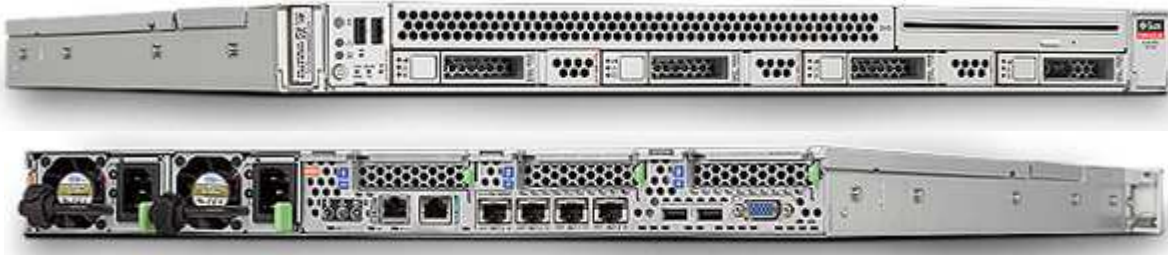
Figure 4 – Sun Server X3-2 (formerly the Sun Fire X4170 M3 server) Front and Rear Panel Ports (Intel-based)
