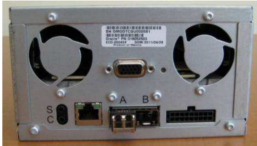
Figure 4 – StorageTek T10000C Tape Drive (Rear)
