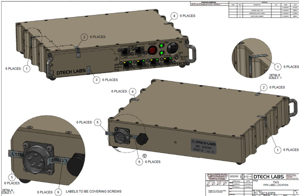
**Figure 7: TXC3-FIPS Tamper Evidence**
