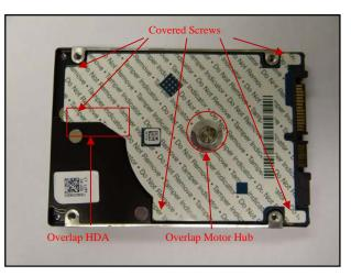
• Security labels on side of drive to provide tamper-evidence of HDA cover removal,
