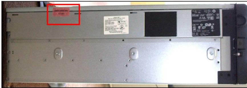
Figure 17 – 4150E Tamper-Evident Seal Application Position (Seal #2)
