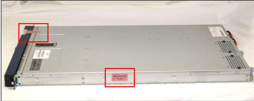
**Figure 13 – 1100E Tamper-Evident Seal Application Positions (Seals #1 and 2)**
