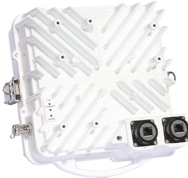
**Figure 7 – Horizon Compact+ Physical Ports**
