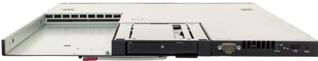
Figure 4 – BladeSystem c3000 Tray with Embedded DDR2 Onboard Administrator
