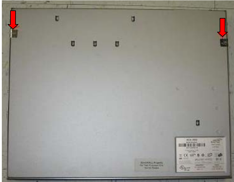
Figure 5: Tamper Evident Seal Locations (Bottom)
