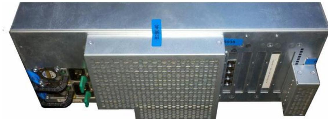
**Figure 6 Installed Louvered Shutters and Tamper-Evident Labels**
