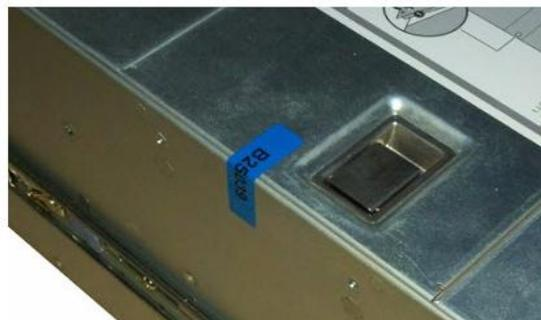
**Figure 14 Tamper-Evident Label Application – Top and Side of Appliance**
