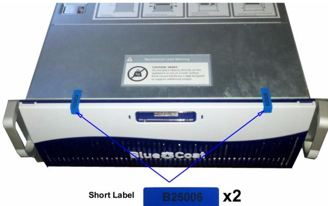
**Figure 15 Front Bezel Label Application Points**
