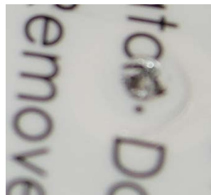
Figure 12: Label (Punctured and Distorted Text)
