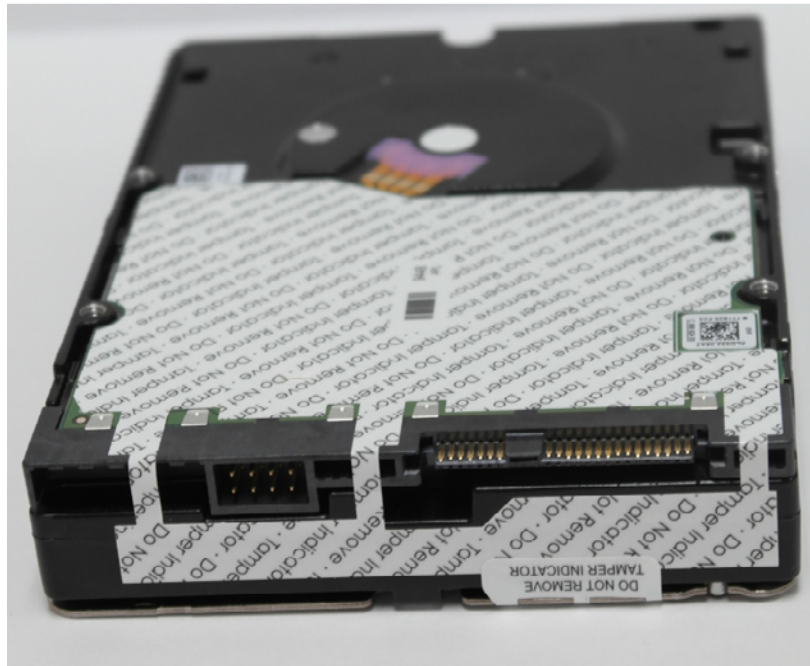
Figure 7: Verdi Module Showing One Overlapping Tamper Label on Connector Side
