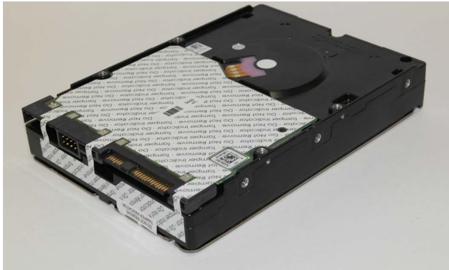
Figure 3: Verdi Module Showing PCBA & Connector Edge Tamper Evidence Label on Underside
