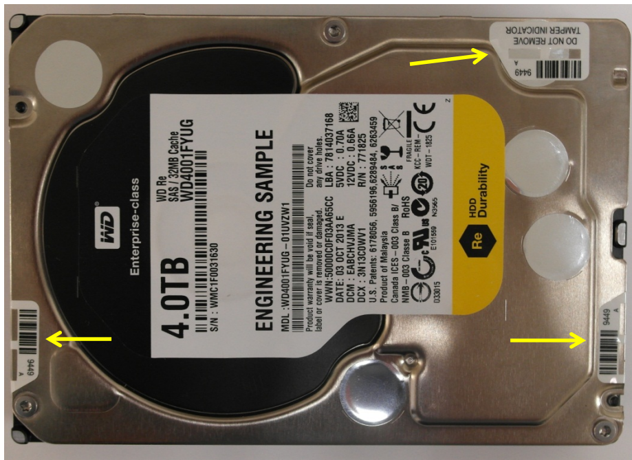
Figure 4: Verdi Module Showing Three (3) Top-Cover Tamper Evidence Labels (See Arrows)
