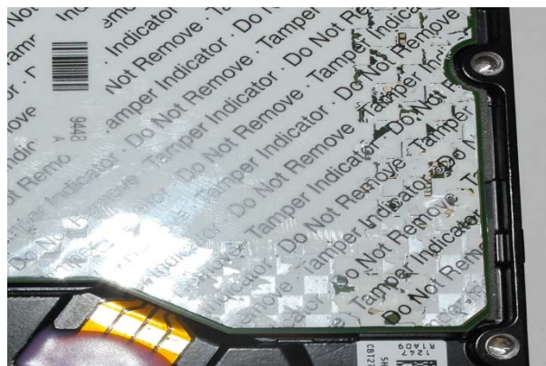
Figure 11: PCBA & Connector Label Showing Signs of Tamper (Reapplied Label)
