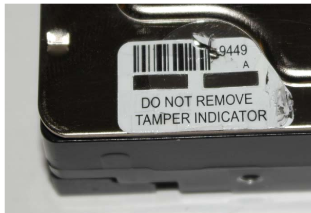
Figure 9: A Top Cover Label Showing Signs of Tamper (Peeling and Cutting)
