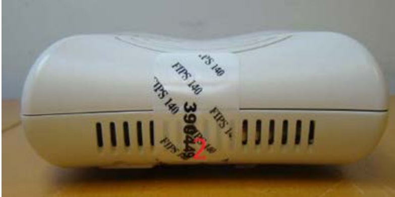
Figure 18 - Aruba AP-105 TEL placement right view
