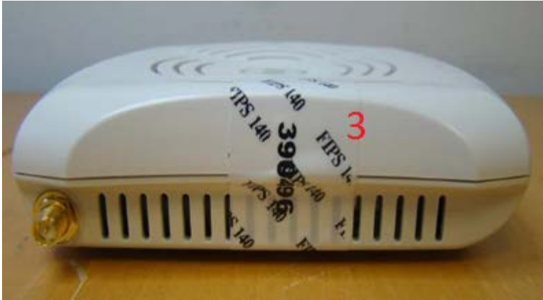
Figure 3 - Aruba AP-92 TEL placement right view
