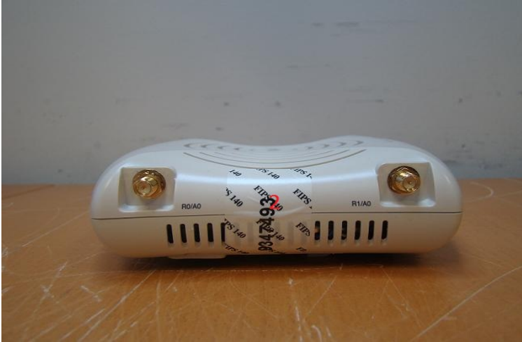
Figure 13 - Aruba AP-104 TEL placement right view
