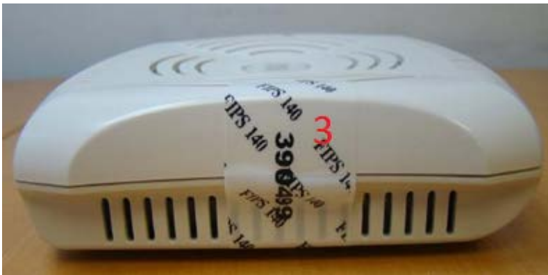
Figure 8 - Aruba AP-93 TEL placement right view
