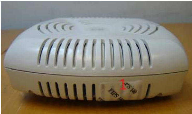
Figure 6 - Aruba AP-93 TEL placement front view
