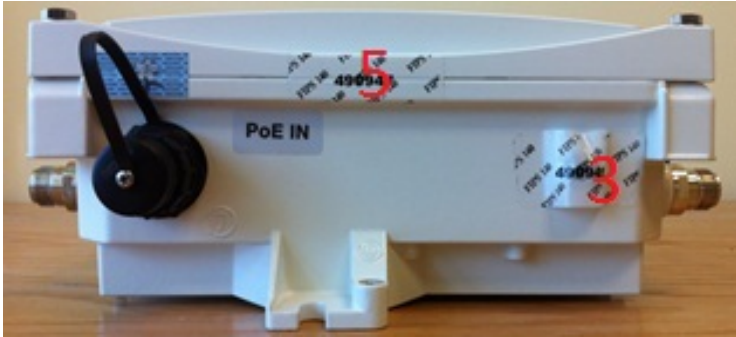
Figure 25 - Aruba AP-175 TEL placement top view
