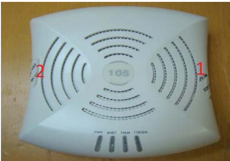
Figure 19 - Aruba AP-105 TEL placement top view
