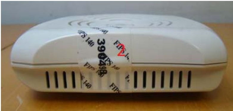
Figure 7 - Aruba AP-93 TEL placement left view
