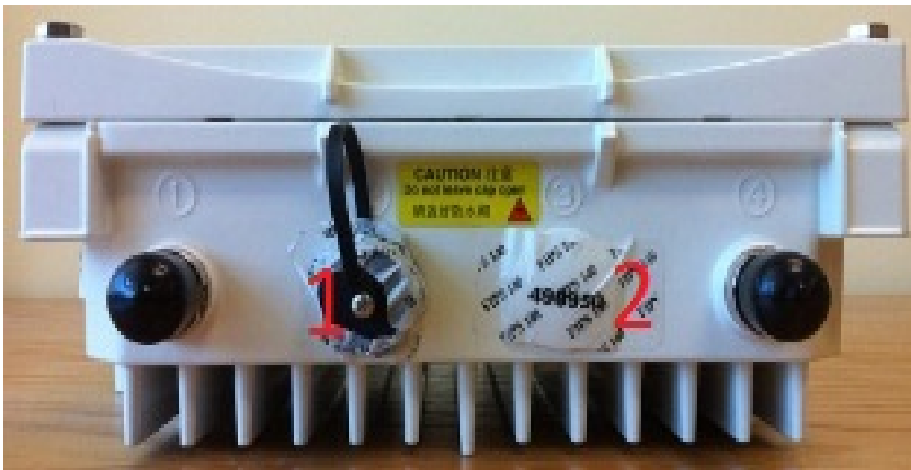
Figure 21 - Aruba AP-175 TEL placement front view
