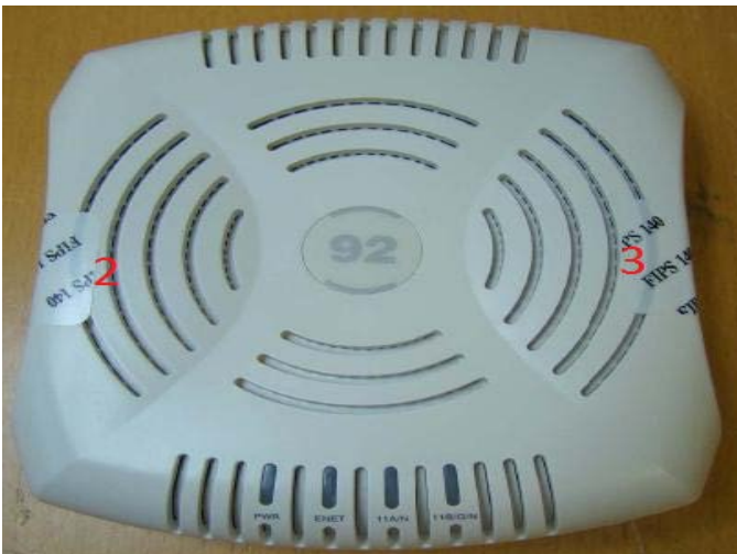
Figure 4 - Aruba AP-92 TEL placement top view
