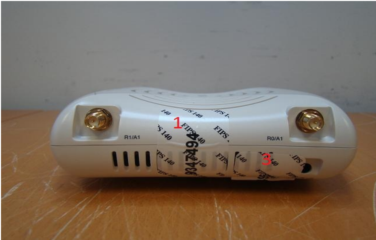
Figure 13 - Aruba AP-104 TEL placement right view
