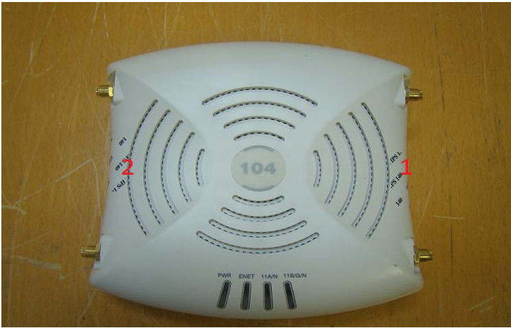
Figure 14 - Aruba AP-104 TEL placement top view
