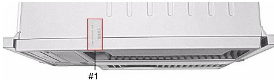
**Figure 25 – 4150F Tamper-Evident Seal Application Position (Front Bezel)**
